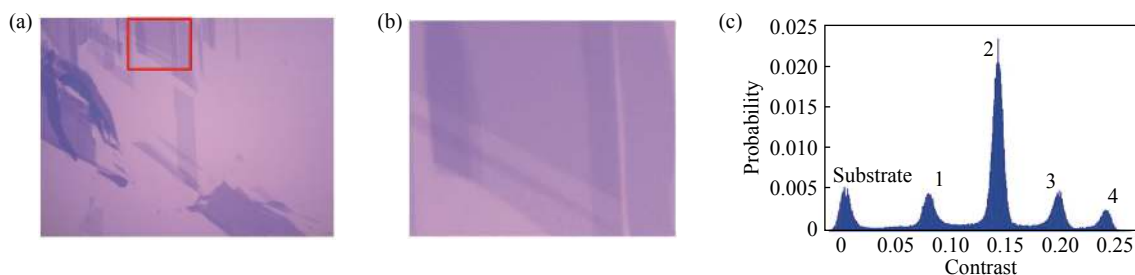
Fig. S3. (Color online) (a) The optical image of mechanical exfoliated graphene. (b) The selected area of the sample (The marked area in (a)). (c) The distribution of G-channel contrast of the selected area.
