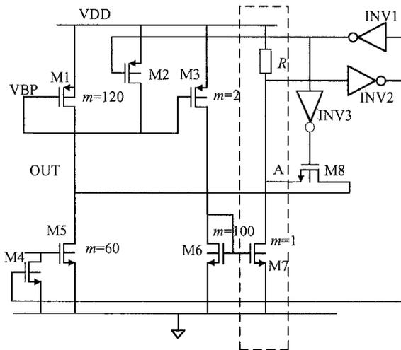
Fig. 3 Over-current protection circuit
