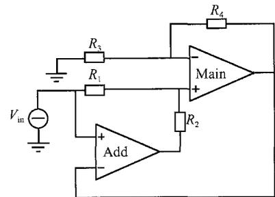
Fig.2 Unity feedback structure of the system-corrected power AMP
