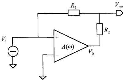
Fig.1 Pre AMP of the system-corrected structure
