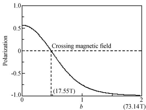
Fig. 5 Linear polarization factor of optical transitions of CdSe quantum rods with  $R = 3\text{nm}$  and  $e = 2$  and  $\Delta_c = 25\text{meV}$  at  $T = 10\text{K}$  as a function of  $b$
