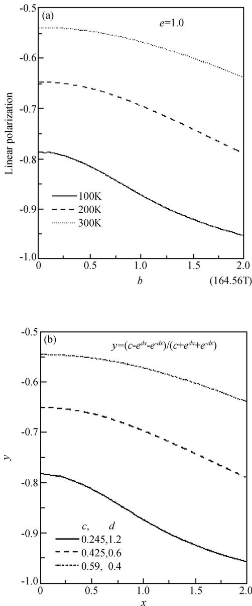
Fig. 3 (a) Linear polarization factors of optical transitions of CdSe quantum spheres with  $R = 2\text{nm}$  and  $\Delta_c = 25\text{meV}$  as functions of  $b$ ; (b) Function  $y = \frac{c - e^{dx} - e^{-dx}}{c + e^{dx} + e^{-dx}}$
