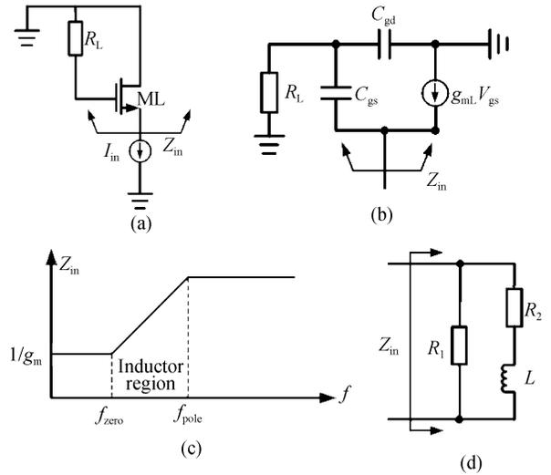
Fig. 4 Active inductor and the equivalent circuit
