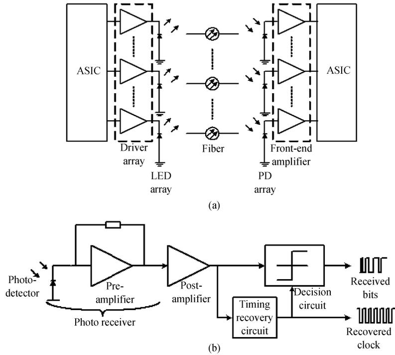
Fig.1 (a) System structure of 12-channel OEIC transceiver; (b) Single channel block diagram of the receiver
