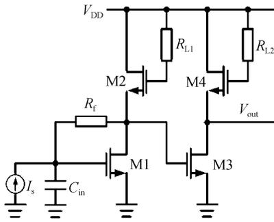
Fig. 3 Schematic of equivalent PD model and TIA circuit
