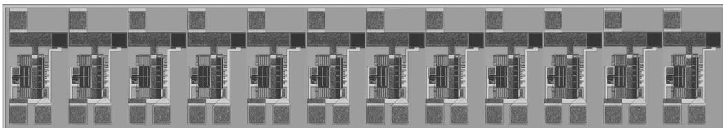
Fig.6 Chip photo of the 12-channels parallel CMOS OEIC receiver
