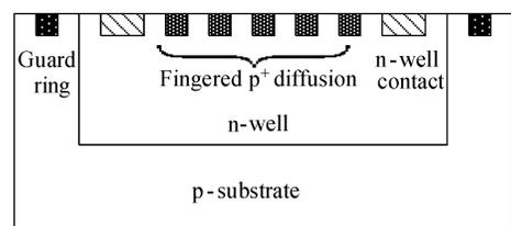
Fig.2 Cross section of the DPD detector structure
