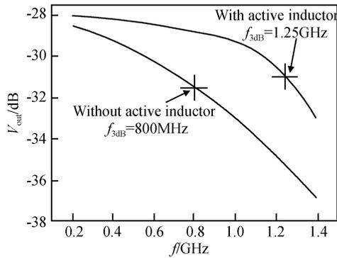
Fig.5 Simulation results of OEIC receiver with and without active inductor
