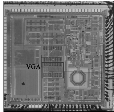
Fig.5 Microphotograph of VGA in SOC
