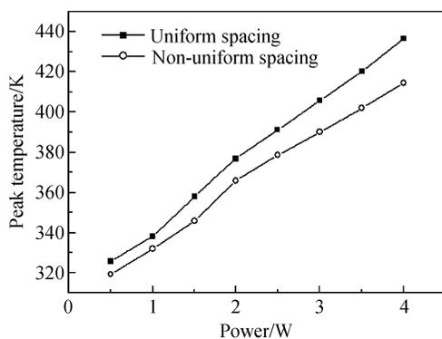
Fig.6 Peak temperature versus power for SiGe HBTs with uniform and non-uniform finger spacing at  $V_{CE} = 5V$
