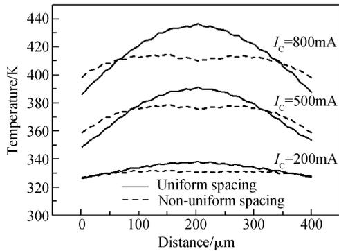
Fig.5 Temperature profile of 20-finger SiGe HBTs with non-uniform and uniform finger spacing
