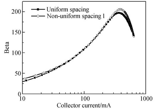
Fig.4 DC current gain versus collector current for HBTs with uniform and non-uniform finger spacing
