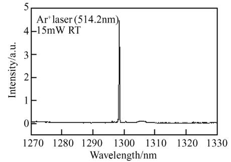
Fig. 1 PL spectrum of a AlGaInAs/AlInAs SQW laser
