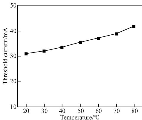
Fig.3 Temperature dependence of threshold current
