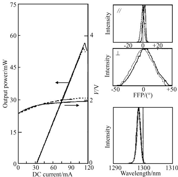
Fig. 2 Output characteristics curves of AlInGaAs/AlInAs LDs at 20°C. Dashed curve shows symmetric wave-guide LDs, and the real curve shows asymmetric wave-guide LDs.
