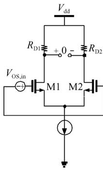
Fig. 1 Resistor loaded differential pair
