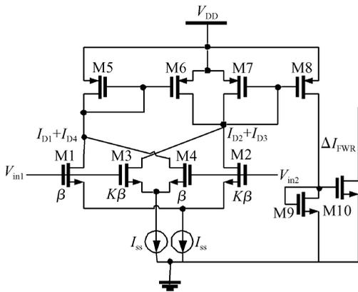
Fig.9 Unbalanced source coupled differential pairs FWR
