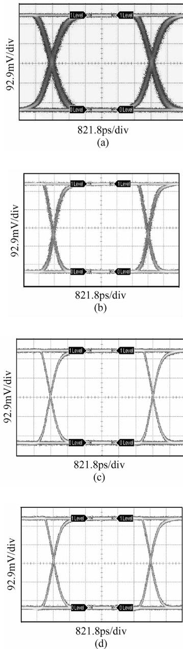
Fig. 11 Measured LA single-end output for input level of 0.5mV (a), 2mV (b), 50mV (c), and 2000mV (d) (Horizontal scale: 821.8ps/div, vertical scale: 92.9mV/div)
