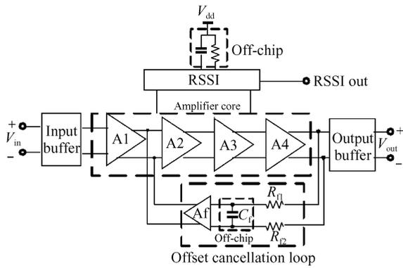
Fig. 3 Limiting amplifier architecture
