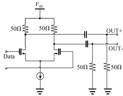
Fig. 5 CML output buffer
