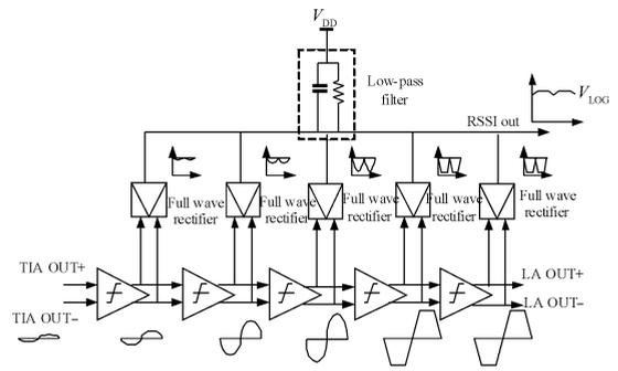
Fig. 2 Block diagram of RSSI
