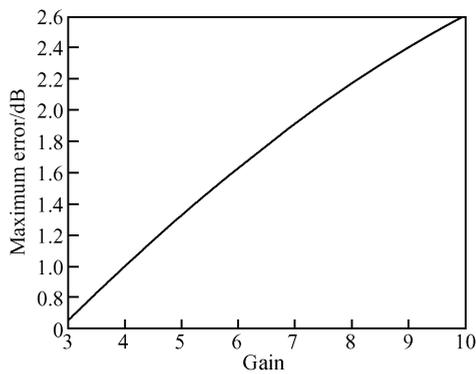
Fig. 6 RSSI maximum error versus each stage gain
