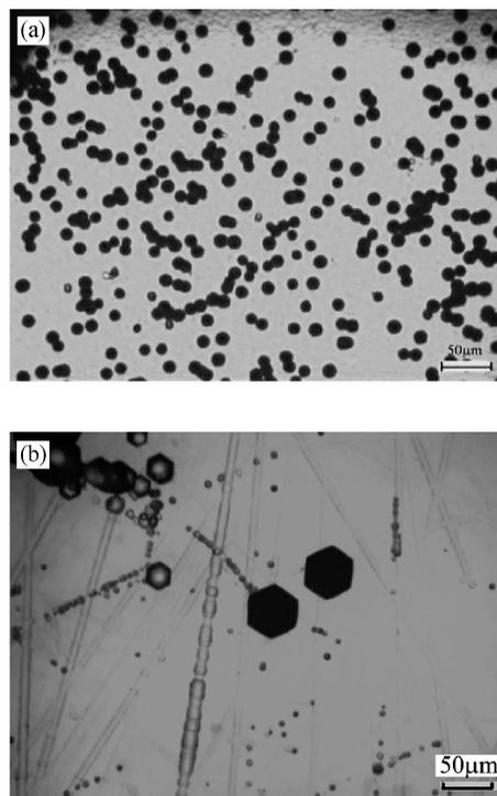
Fig.1 Typical micrographs of etching pattern on the C face (a) and the Si face (b) of 6H-SiC
