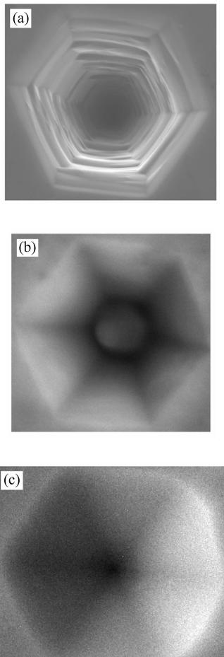
Fig.3 SEM images of KOH etched SiC crystal surface (a) MP; (b) SD etch pit; (c) ED etch pit
