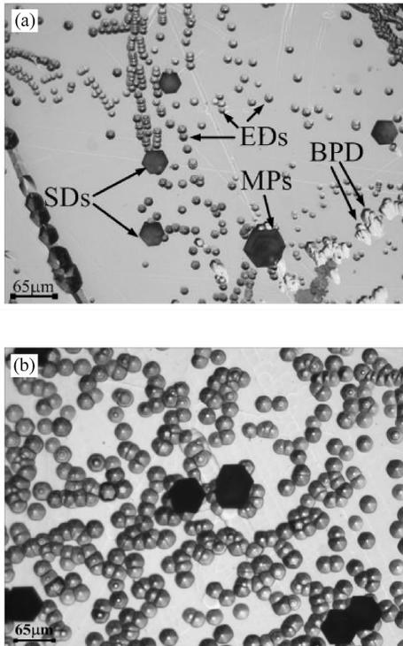
Fig.2 Optical microscope images of sample A (a), sample B (b) on (0001) Si face
