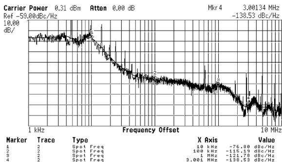
Fig. 9 PLL phase noise at 434.6 MHz
