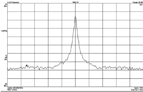
Fig. 8 PLL output spectrum at 434.6 MHz
