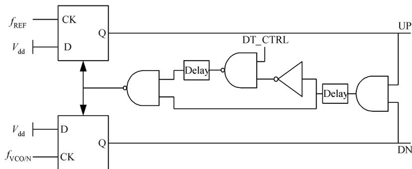
Fig. 5 Block diagram of PFD
