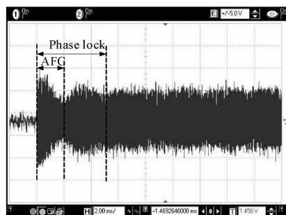
Fig. 7 Control voltage of VCO
