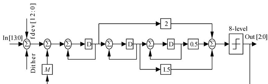
Fig. 4 Block diagram of the 3bit third-order SDM
