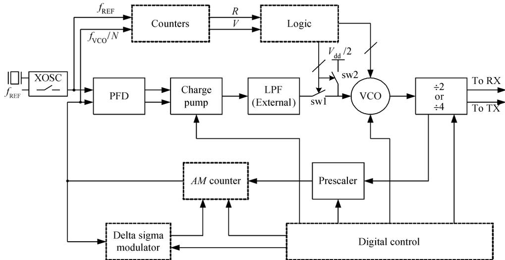
Fig. 1 Frequency synthesizer block diagram
