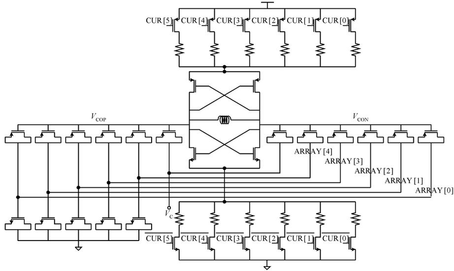
Fig.2 Schematic of VCO
