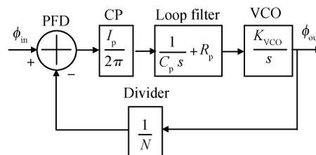
Fig.1 Linear model of a second order charge pump PLL
