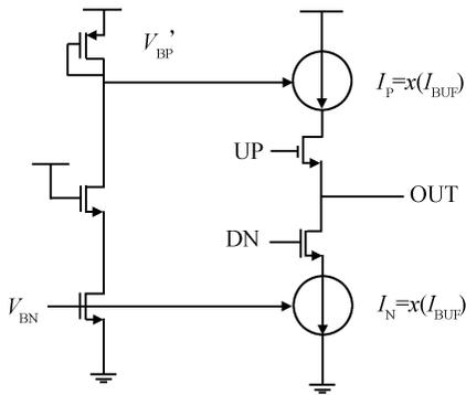
Fig. 4 Charge pump circuit
