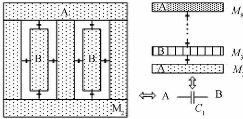
Fig. 7 Metal parasitic capacitance
