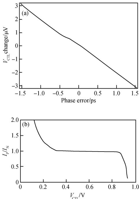
Fig.5 (a) Relationship between  $V_{CTL}$  change and phase error; (b)  $I_P/I_N$  changes with  $V_{CTL}$
