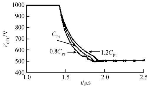
Fig. 8 Transient simulation results of the  $V_{CTL}$  signal
