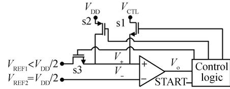
Fig. 10 Startup circuit
