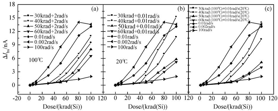
Fig.1  $I_{bs}$  of LM108 versus the total dose at various dose-rate switching methods (a) 1st method; (b) 2nd method; (c) 3rd method
