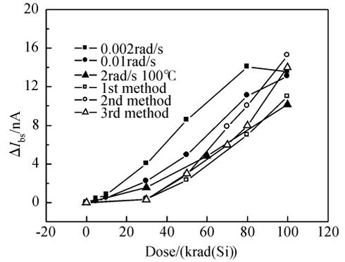
Fig. 3  $I_{bs}$  of LM108 versus different radiation methods
