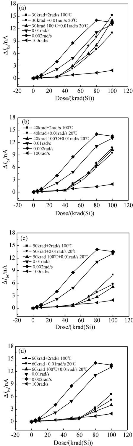
Fig. 2  $I_{bs}$  of LM108 versus the total dose at the same switching dose and different irradiation methods
