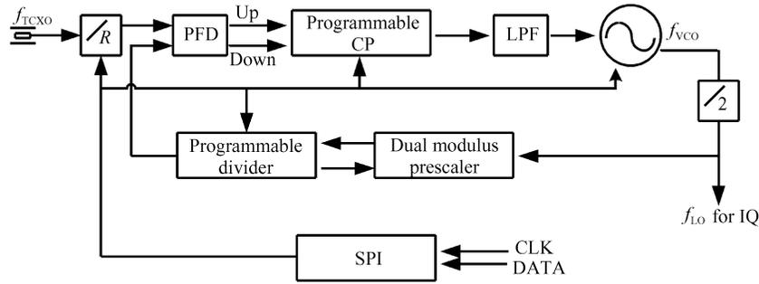
Fig.1 Block diagram of the implemented frequency synthesizer
