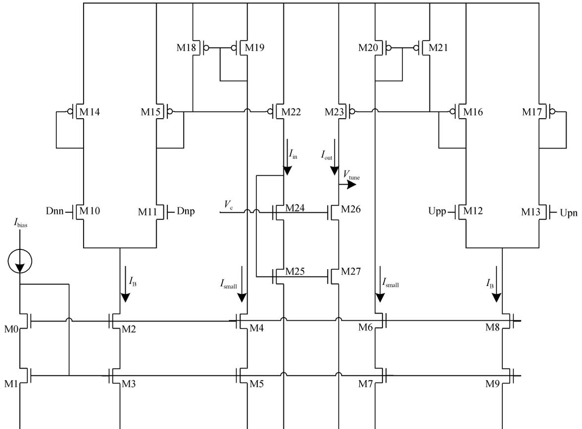
Fig. 5 Charge pump circuit
