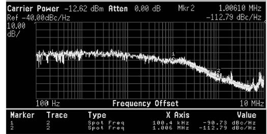
Fig.8 Measured PLL phase noise
