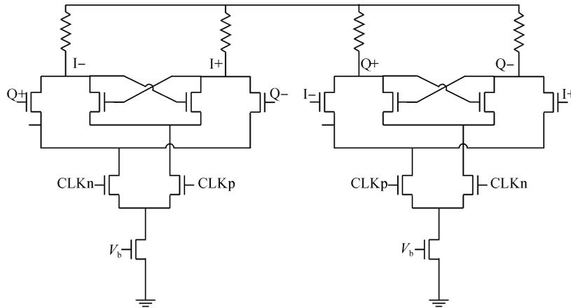
Fig. 3 High frequency divide-by-two circuit
