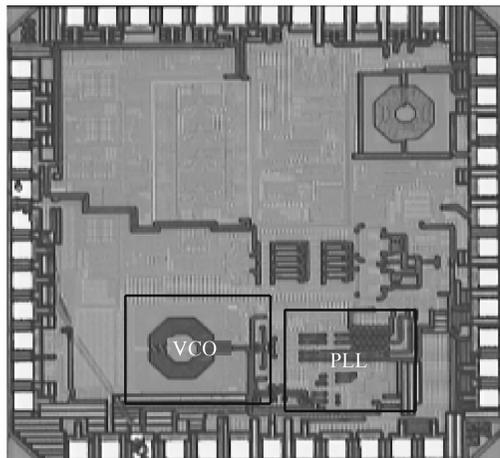
Fig.7 Die microphotograph of the complete CMOS receiver front end
