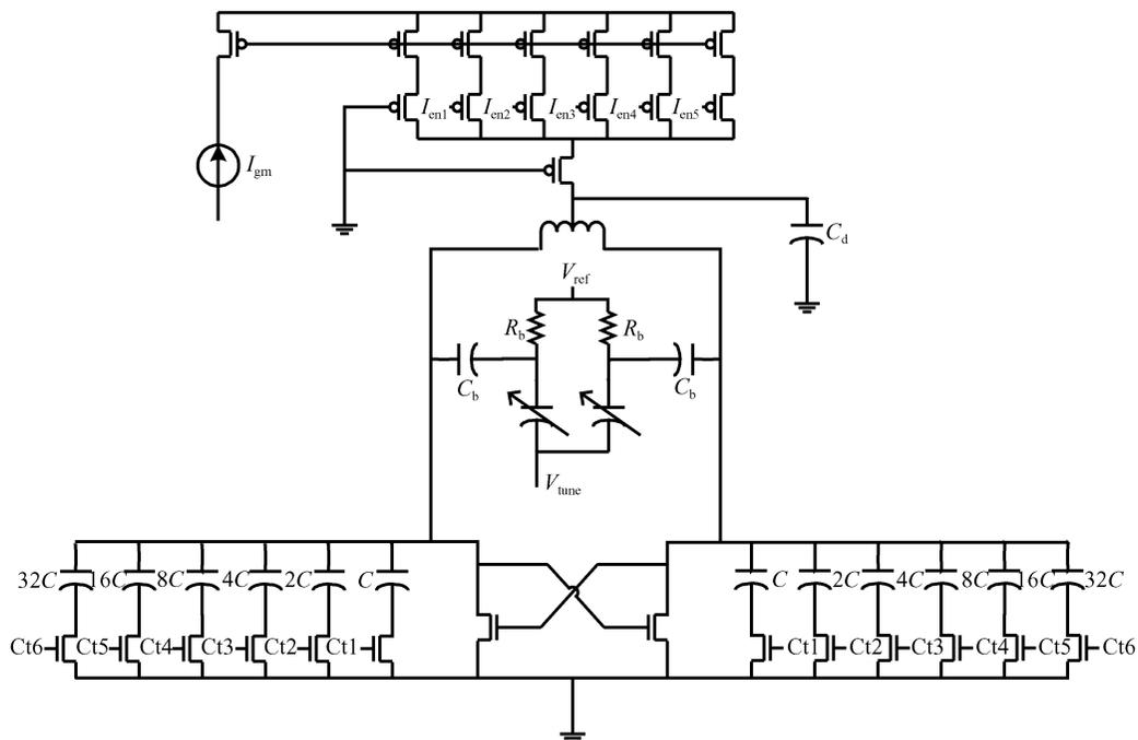
Fig.2 Diagram of the proposed wide-band VCO
