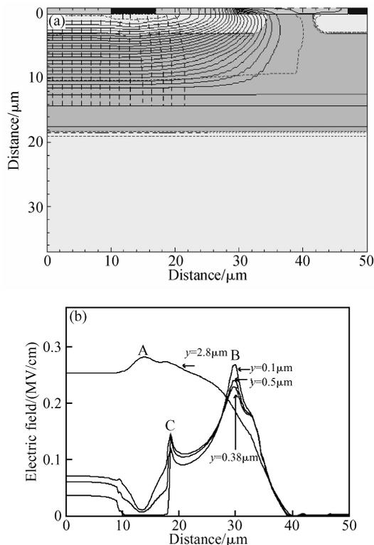
Fig. 2 Electronic solutions for the structure in Fig. 1 (a) Electrical potential distribution; (b) Electric field intensity
