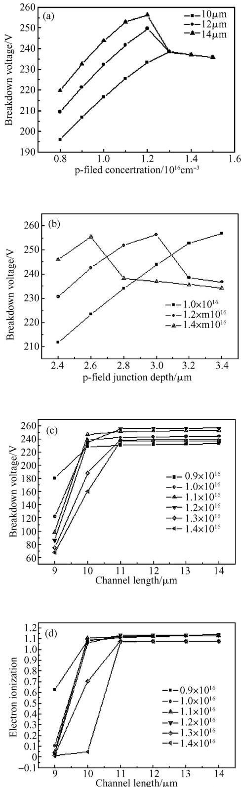
Fig.4 Structure parameters of drift and channel (a) Breakdown voltage  $V_{br}$  versus drift concentration  $C_{dt}$ ; (b)  $V_{br}$  versus drift junction depth  $J_{dt}$ ; (c)  $V_{br}$  versus channel length  $L_{ch}$ ; (d) Electron ionization  $\int \alpha_e$  versus  $L_{ch}$
