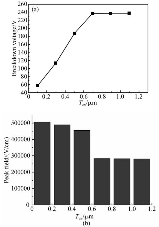
Fig.5 Influence of field-oxide thickness ( $T_{ox}$ ) on the device (a)  $V_{br}$  versus  $T_{ox}$ ; (b)  $E_m$  versus  $T_{ox}$
