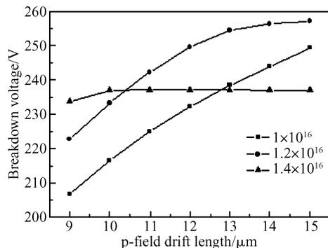
Fig. 3  $V_{br}$  versus  $L_{dt}$   $L_{ch} = 14\mu\text{m}$ ,  $J_{dt} = 14\mu\text{m}$
