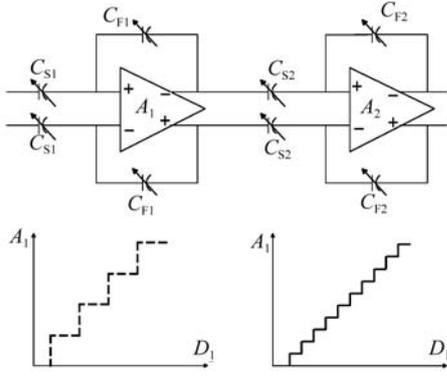
Fig.1. Two stages pipeline PGA system.
