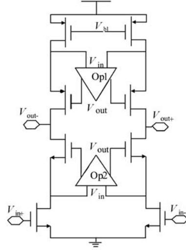
Fig.3. Schematic of operational amplifier.
