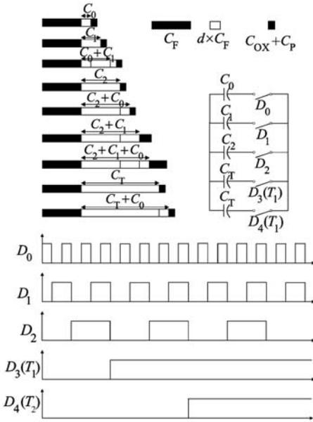
Fig.4. Mixed coding of thermometer and binary.
