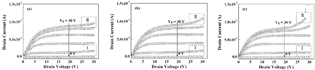
Fig. 6. Measured output characteristics of different samples: (a) SA1; (b) SA2; (c) SA3. The regions I and II correspond to the first peak and second peak substrate current, respectively.
