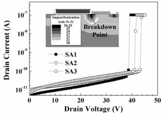
Fig. 7. Measured drain current versus drain voltage curves at  $V_g = 0$  of samples SA1, SA2 and SA3.
