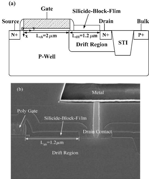
Fig. 1. Device structure of an n-channel DEMOS transistor: (a) Cross-section schematic; (b) SEM image of real structure.
