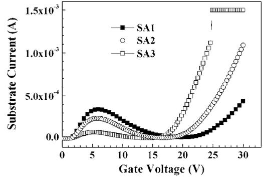
Fig. 5. Measured substrate current versus gate voltage curves at  $V_d = 30$  V of samples SA1, SA2 and SA3.
