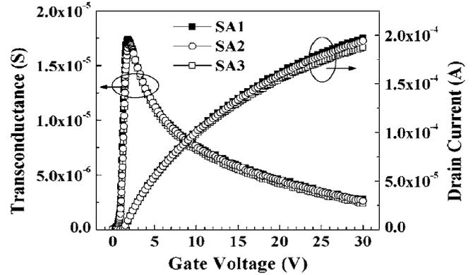
Fig. 2. Measured transconductance and drain current versus gate voltage curves at  $V_d = 0.1$  V of samples SA1, SA2 and SA3.
