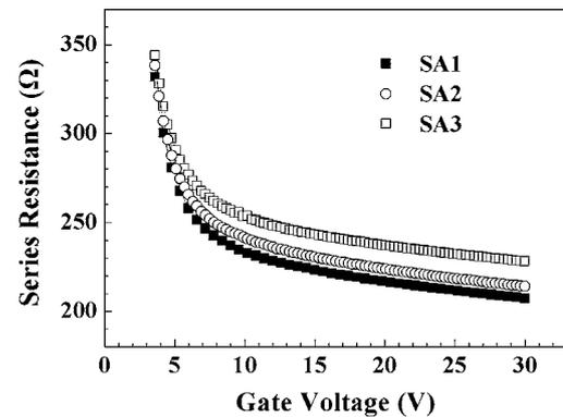
Fig. 3. Extracted source/drain series resistance versus gate voltage curves of samples SA1, SA2 and SA3.
