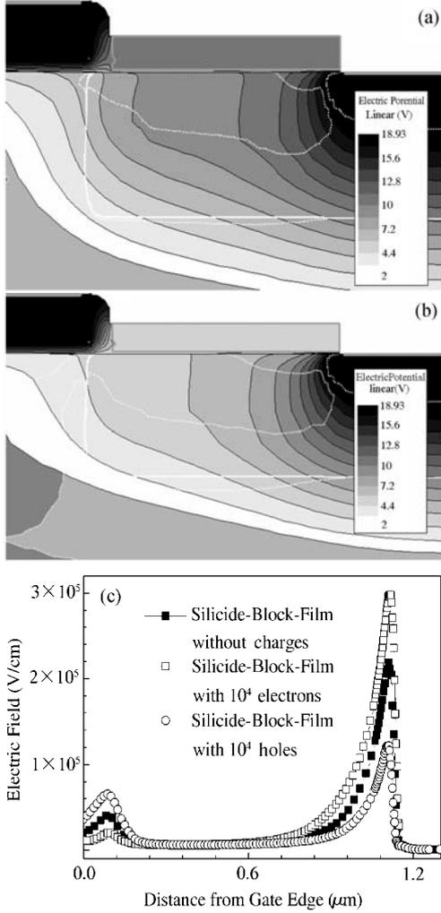
Fig. 4. Electric potential and electric field distribution with different block films under  $V_d = V_g = 30$  V: (a) Electric potential contours with block film containing no charges; (b) Electric potential contours with block film containing  $1 \times 10^4$  electrons; (c) Electric field distribution along the drift region with block film containing no charges,  $1 \times 10^4$  electrons or holes.
