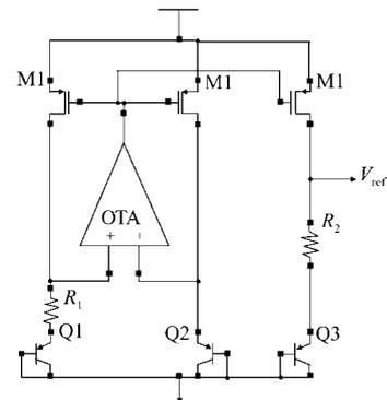
Fig. 1. Typical CMOS BGR.
