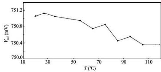
Fig. 5.  $V_{ref}$  variation with temperature.
