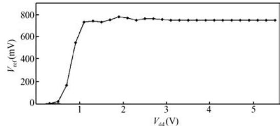
Fig. 6.  $V_{ref}$  variation with supply voltage.
