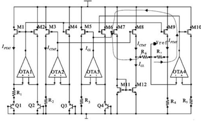
Fig. 2. Bandgap reference circuit.
