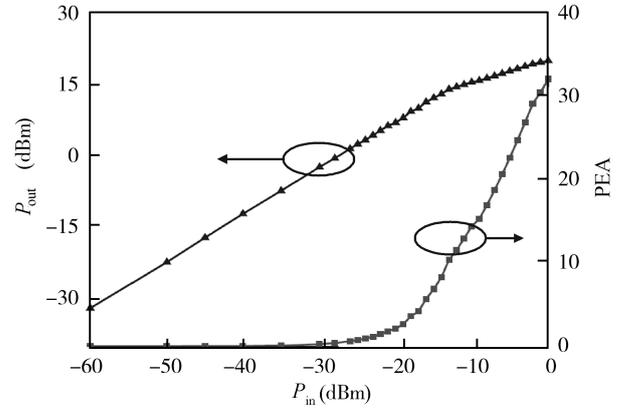
Fig. 9. Output power ( $P_{out}$ ) and power-added efficiency (PAE) versus input power ( $P_{in}$ ) of the PA.
