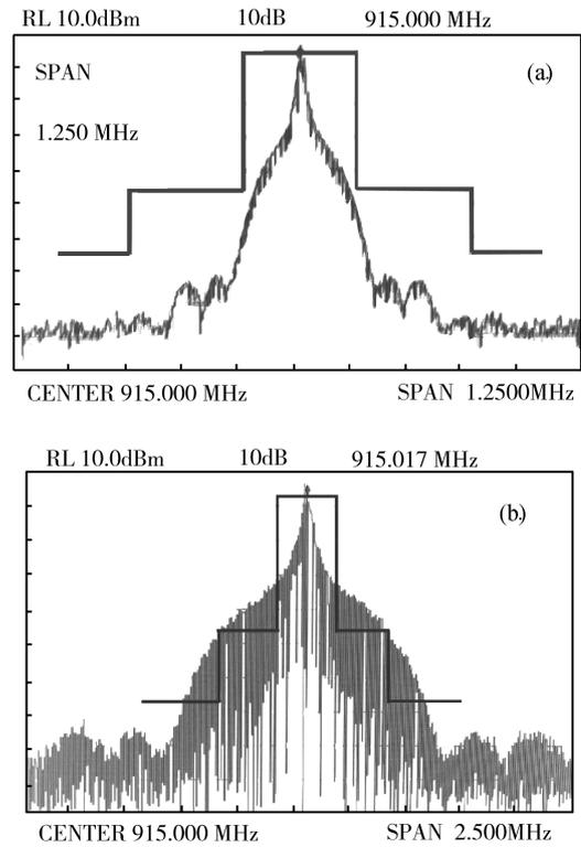
Fig. 10. Signal spectra of different data rates: (a) 10 kbps; (b) 40 kbps.
