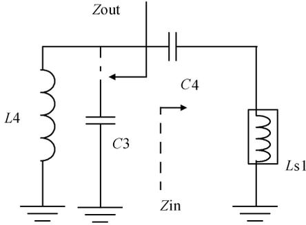
Fig. 2. Equivalent circuit of the inter-stage matching networks.
