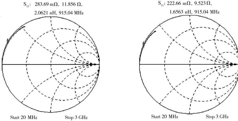
Fig. 4. S-parameter of a bondwire and its mutual inductance.
