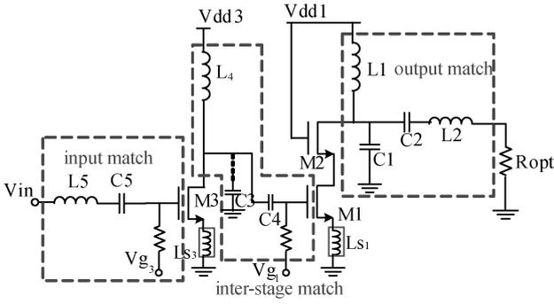
Fig. 1. Matching networks of class-E PA.
