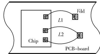
Fig. 6. Implementation of  $L_1$  and  $L_2$  with bondwires.
