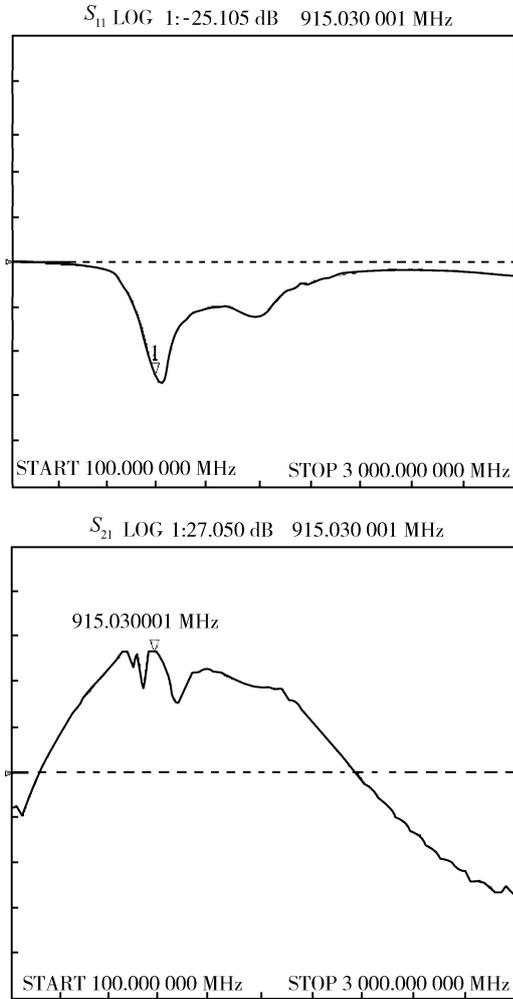
Fig. 8. Measured  $S$ -parameters ( $S_{11}$ ,  $S_{21}$ ) of the PA.
