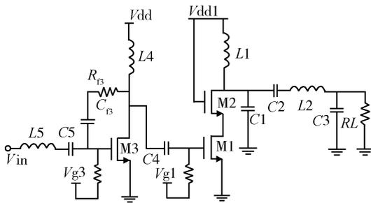
Fig. 5. Schematic of the class-E power amplifier.
