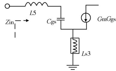
Fig. 3. Equivalent circuit of the input matching networks.
