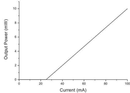
Fig.5. Typical  $L-I$  characteristics of the device at RT.
