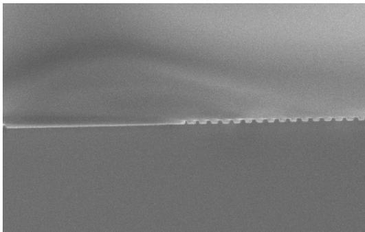
Fig.3. SEM photograph of the sampled grating.
