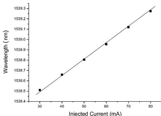
Fig.7. Current-dependent wavelength of the laser at RT.
