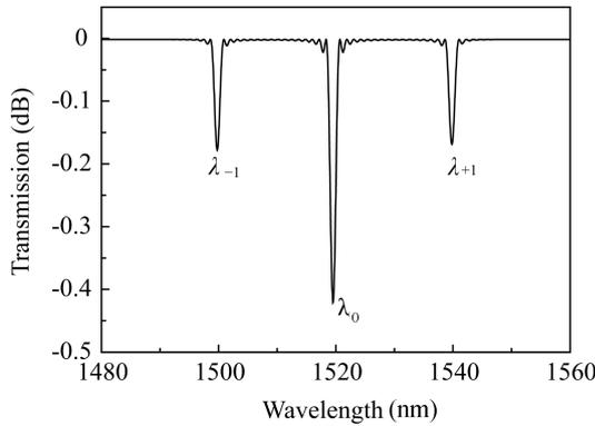
Fig.2. Calculated transmission spectrum of the designed sampled grating.
