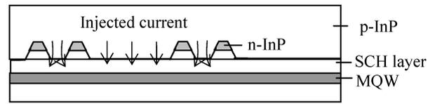
Fig.4. Schematic illustration of the sampled grating.
