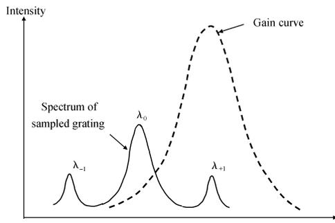
Fig.1. Schematic spectra of the gain curve and sampled grating.
