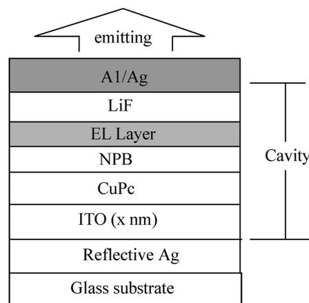
Fig. 1. Schematic structure of the microcavity OLED.
