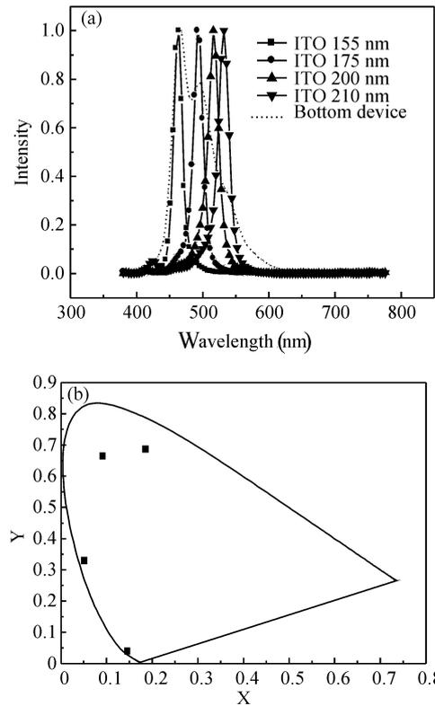
Fig. 3. (a) TBADN:DSAPh EL spectra with four different thicknesses of ITO (the dotted line represents EL spectra of bottom emitting device) and (b) CIE<sub>x,y</sub> coordinates with four different thicknesses of ITO.
