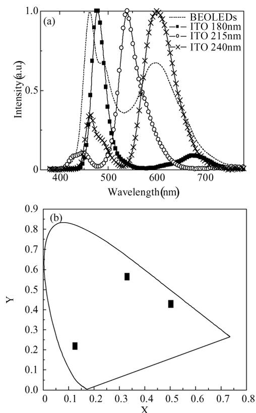
Fig. 4. (a) “Alq<sub>3</sub>:DCJTb/TBADN:TBPe/Alq<sub>3</sub>:C545” device EL spectra with four different thicknesses of ITO (and the dotted line represents EL spectra of bottom emitting device) and (b) CIE<sub>x,y</sub> coordinates with four different thicknesses of ITO.
