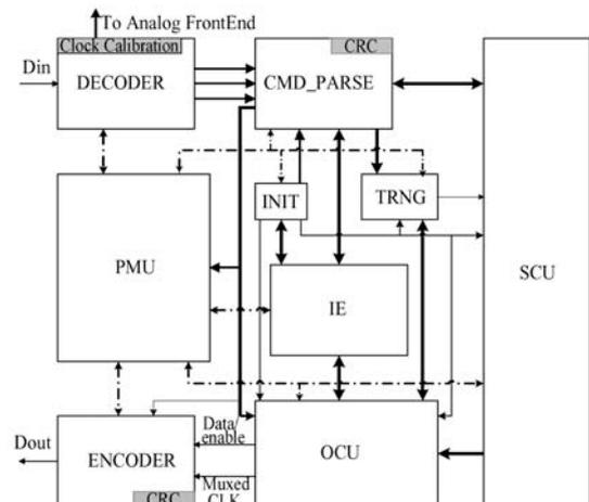
Fig. 1. Architecture of the digital processor. DECODER: PIE decoder unit; CMD\_PARSE: command parse unit; PMU: power management unit; INIT: initiation unit; TRNG: true random number generator; SCU: state control unit; IE: interface to EEPROM; ENCODER: unit for encoding; OCU: output control unit.
