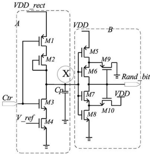
Fig. 6. Analog part of the TRNG.
