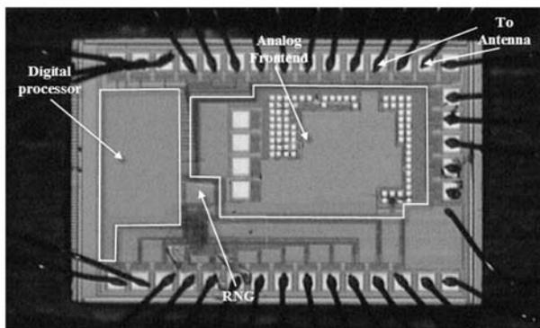
Fig. 9. Micrograph of the RFID tag chip.
