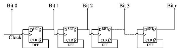
Fig. 5. Structure of the ripple counter.
