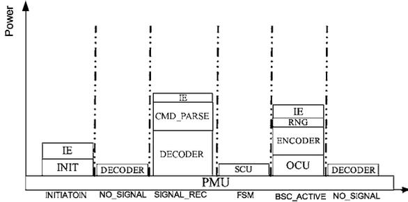
Fig. 3. Power management of the digital processor at system level.
