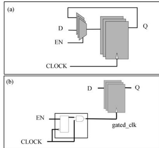
Fig. 4. Reduction of activity by clock gating: (a) Circuit with high activity; (b) Circuit with low activity.
