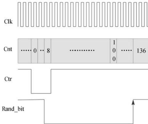
Fig. 7. Operation of the TRNG.
