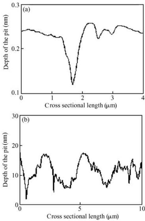
Fig. 4. Cross-sectional of AFM for *a*-plane GaN with (a) the low-temperature GaN as buffer layer and (b) the high-temperature AlN as buffer layer.
