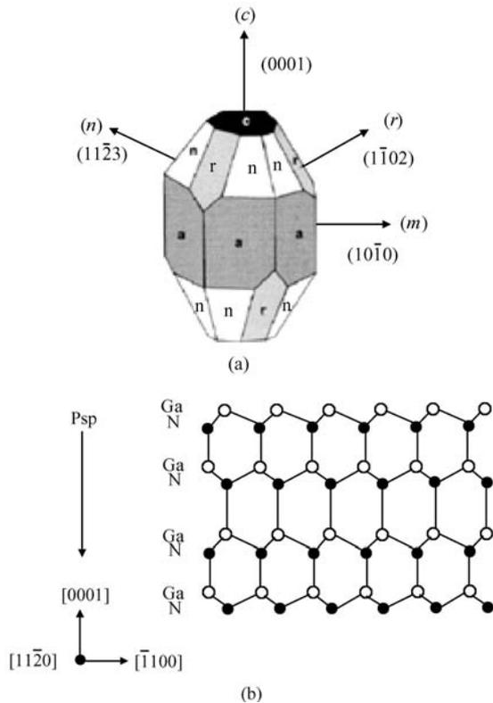
Fig. 2. Schematic representations of (a) the epitaxial relationship between the *r*-plane sapphire substrate of the *a*-plane GaN film and (b) the plan view of the surface atoms which lie on the *a*-plane GaN surface.
