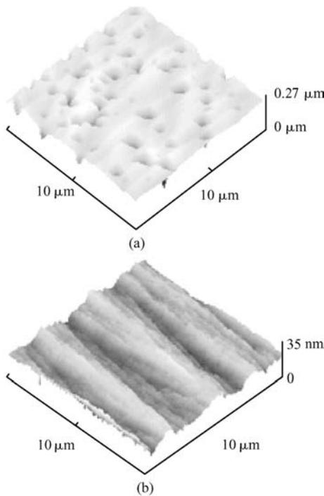
Fig. 5. 3D view of AFM for *a*-plane GaN with (a) the low-temperature GaN as buffer layer and (b) the high-temperature AlN as buffer layer.
