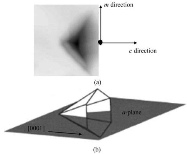
Fig. 6. (a) Surface morphology measurements of *a*-plane GaN with  $1 \times 1 \mu\text{m}^2$  AFM; (b) V defect, shown schematically, which is commonly observed in *c*-plane growth.
