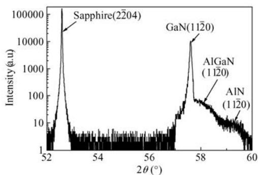
Fig. 8. XRD spectra using  $2\theta-\omega$  scan for modulate buffer.
