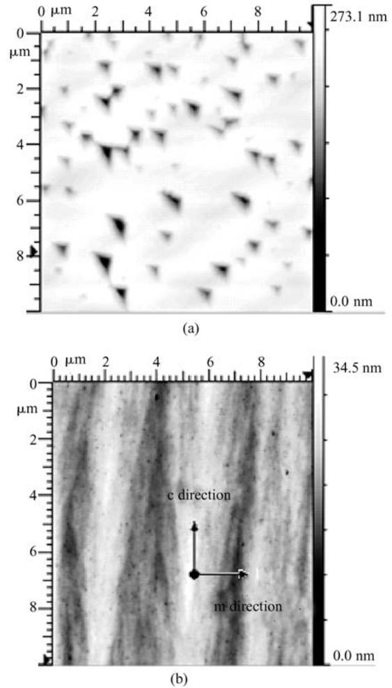
Fig. 3. Surface morphology of AFM for *a*-plane GaN (a) with the low-temperature GaN buffer layer and (b) with the high-temperature AlN buffer layer.
