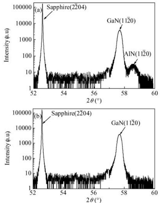
Fig. 7. XRD spectra using  $2\theta-\omega$  scan for (a) *a*-plane GaN grown with HT AlN buffer layer on *r*-plane  $[1\bar{1}02]$  sapphire and (b) *a*-plane GaN grown with LT GaN buffer layer on *r*-plane  $[1\bar{1}02]$  sapphire.
