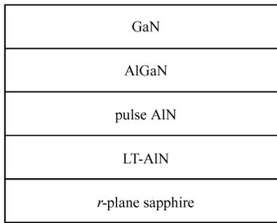
Fig. 1. Schematic representations of the new structure.
