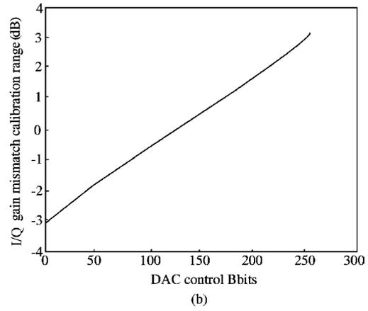
Fig. 6. (a) *I/Q* phase calibration range; (b) *I/Q* gain calibration range.
