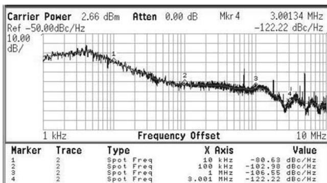
Fig. 14. PLL phase noise at 434.6 MHz.
