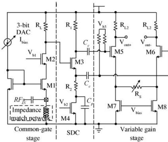
Fig. 2. Circuit of the wideband LNA.
