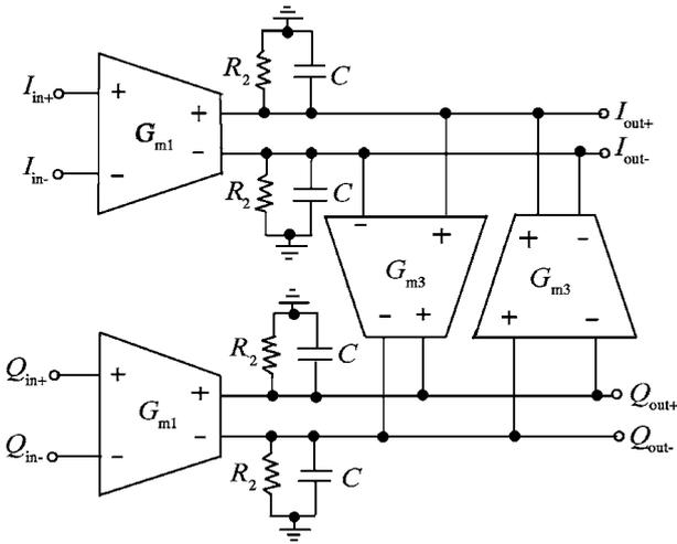
Fig. 7. Block diagram of one stage polyphase filter.
