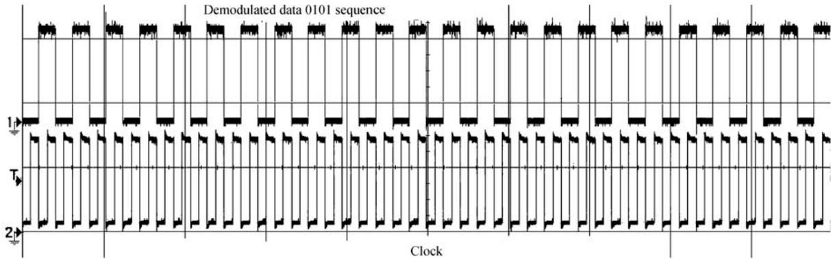
Fig. 12. Demodulated waveform at 4.8 kps data rate.
