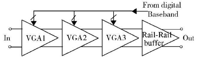
Fig. 8. Block diagram of VGA.
