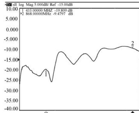
Fig. 11. Measured input return loss of the receiver.
