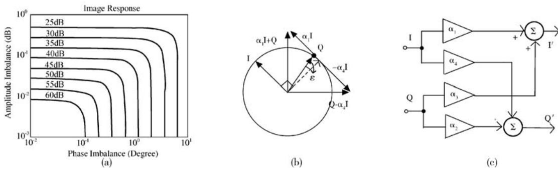
Fig. 4. Phase imbalance calibration structure: (a) Image responses versus amplitude and phase imbalance; (b) Special condition:  $\beta_1$  and  $\alpha_2$  equals to one; (c) Practical implementation.
