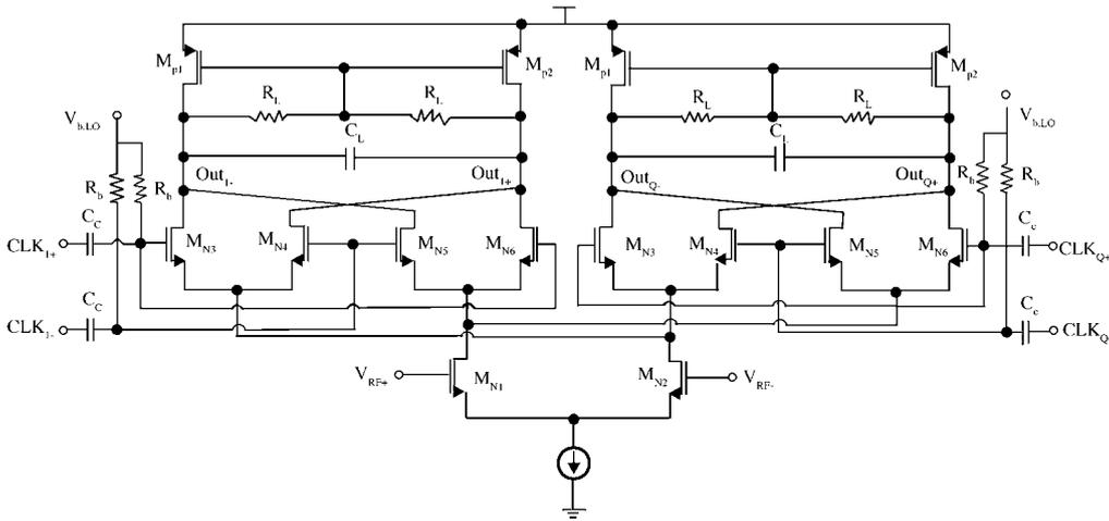
Fig. 3. Schematic of quadrature down-converter.
