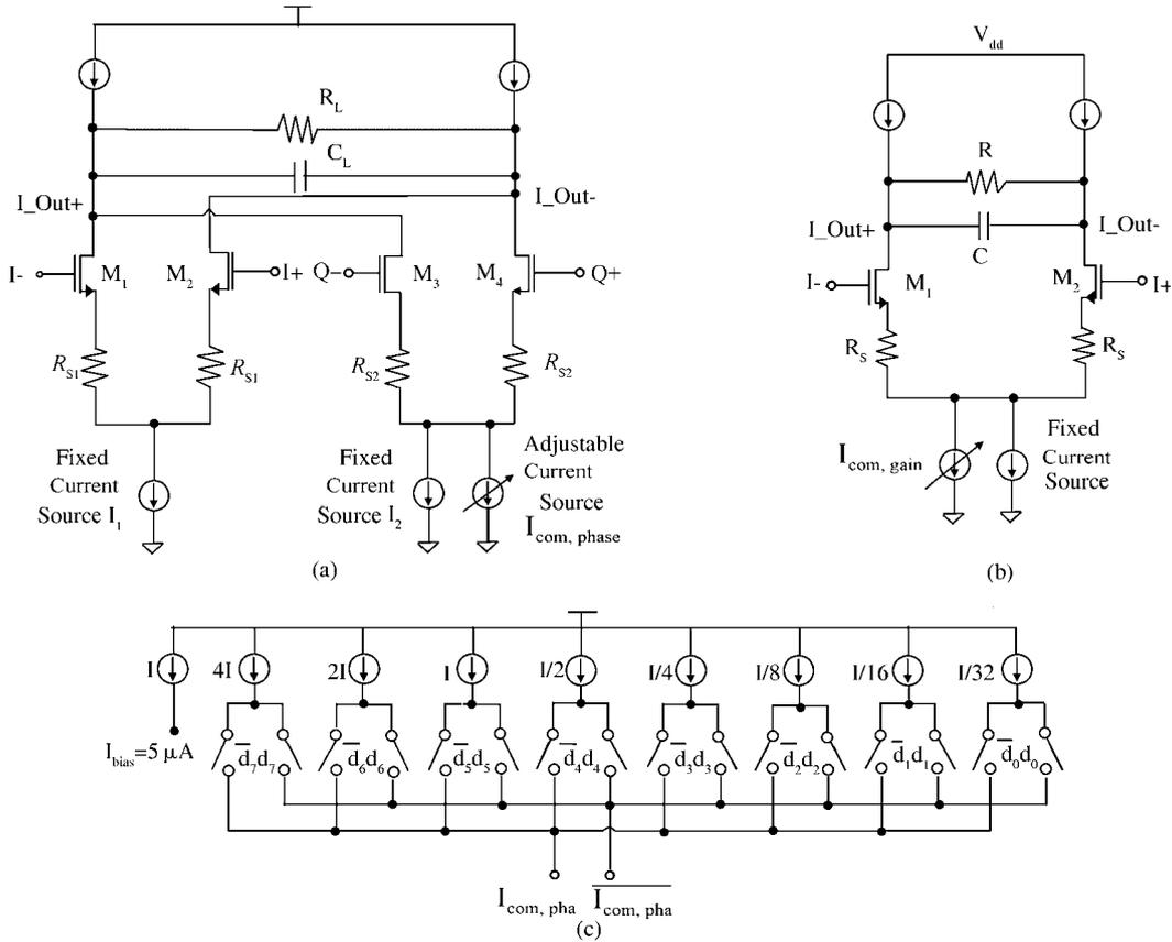
Fig. 5. (a) Schematic of phase imbalance compensation; (b) Schematic of gain imbalance compensation; (c) Current steering 8-bit DAC.
