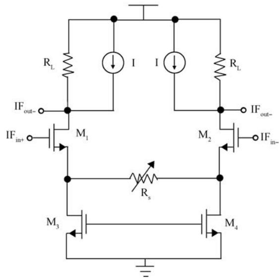
Fig. 9. Schematic of VGA.
