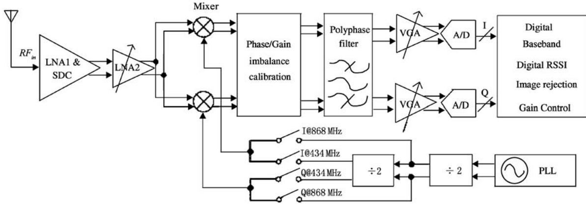
Fig. 1. Receiver block diagram.
