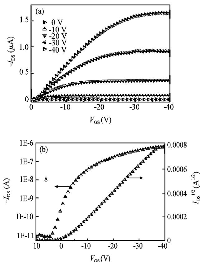
Fig. 4. Drain output and transfer characteristics of the bilayer OFET after 3 months in a continuous air environment.
