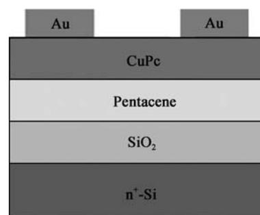
Fig. 1. Schematic diagram of the top-contact bilayer OFET.
