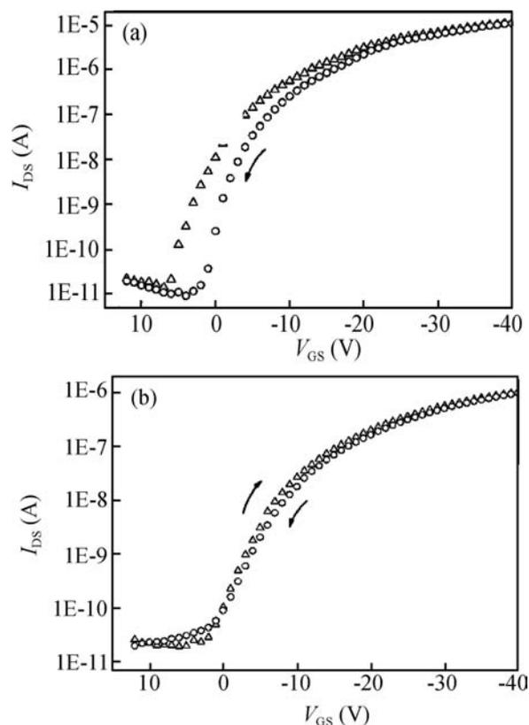
Fig. 5. Transfer characteristics of pentacene-based OFETs (a) without and (b) with the CuPc protecting layer in air after a period of 3 months.
