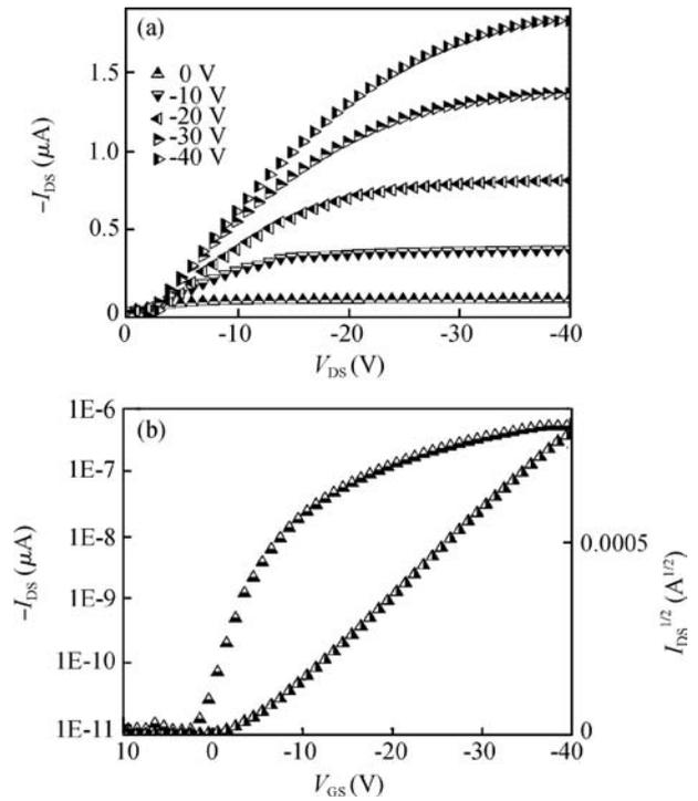
Fig. 3. Drain output and transfer characteristics of the bilayer OFET.
