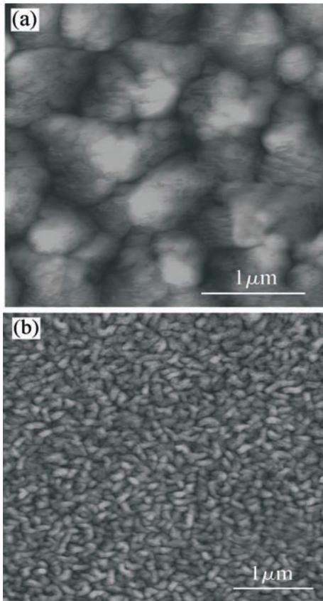
Fig. 2. AFM images of (a) pentacene and (b) CuPc.
