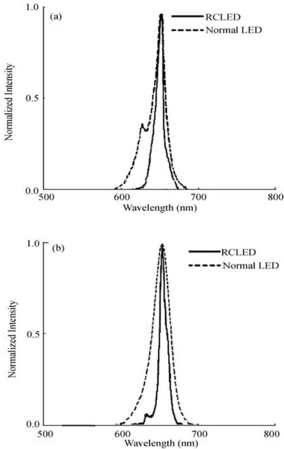
Fig. 3. (a) PL spectrum and (b) EL spectrum of the RCLED and the normal LED.
