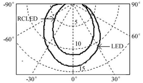
Fig. 4. Far-field strength as a function of angle of the RCLED and the traditional LED.
