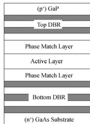
Fig. 1. Schematic structure of the RCLED.
