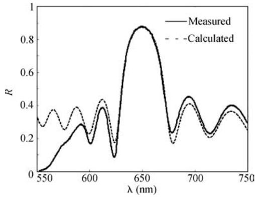
Fig. 2. Calculated and measured reflection spectrum of 15 pairs of AlGaInP/GaInP DBRs.
