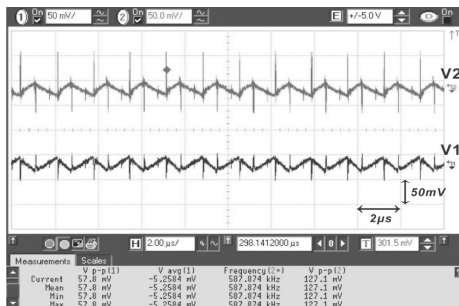
Fig. 13. Ripples of two output voltages.
