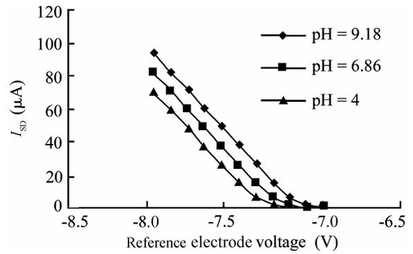
Fig. 6. Input characteristic in different pH solutions.
