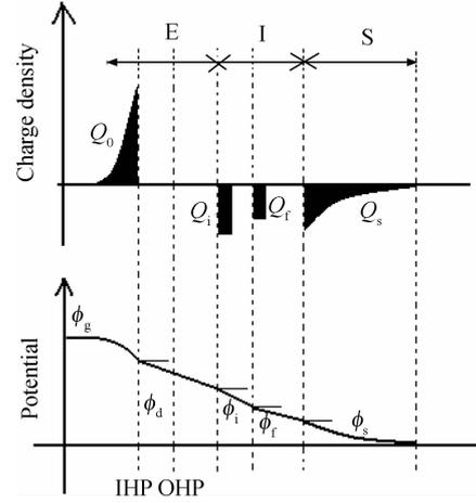
Fig. 2. Charges and potential profiles of a CMOS MFGFET system.
