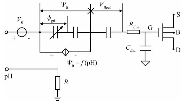
Fig. 3. Equivalent electric circuit of the MFGFET structure.
