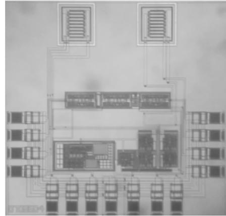
Fig. 7. Photo of the MFGFET pH sensor.
