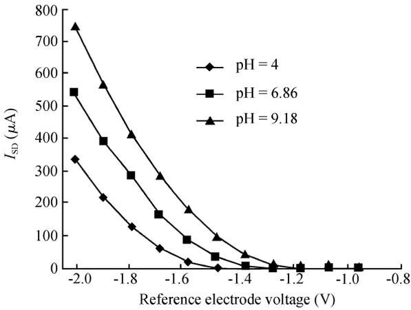
Fig. 5. Simulation results of input characteristic of the MFGFET (PMOS) when  $Q_f = 0$ .
