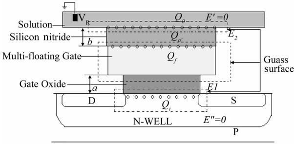
Fig. 1. Effective model of the CMOS MFGFET.
