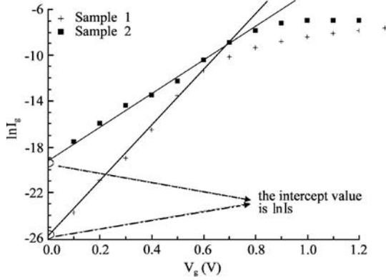
Fig. 5. Plot of  $\ln I_g$  as a function of  $V_g$  derived from the forward-biased  $I_g$ - $V_g$  Schottky characteristic of Fig. 3(b).
