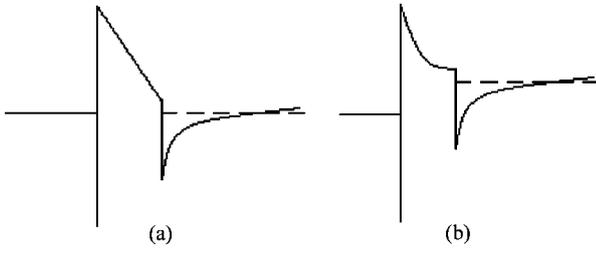
Fig. 4. Comparison of the energy band structure change (a) before and (b) after gate recess etching.
