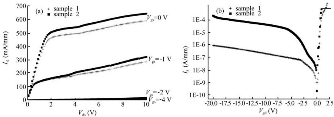
Fig. 3. (a) Comparison of the  $I_d$ - $V_{ds}$  characteristics of sample 1 and sample 2, with  $V_{gs}$  varied from  $-4$  to  $0$  V (step width:  $1$  V); (b) Comparison of the  $I_g$ - $V_{gd}$  characteristics of sample 1 and sample 2, with  $V_{gd}$  varied from  $-20$  to  $2$  V.
