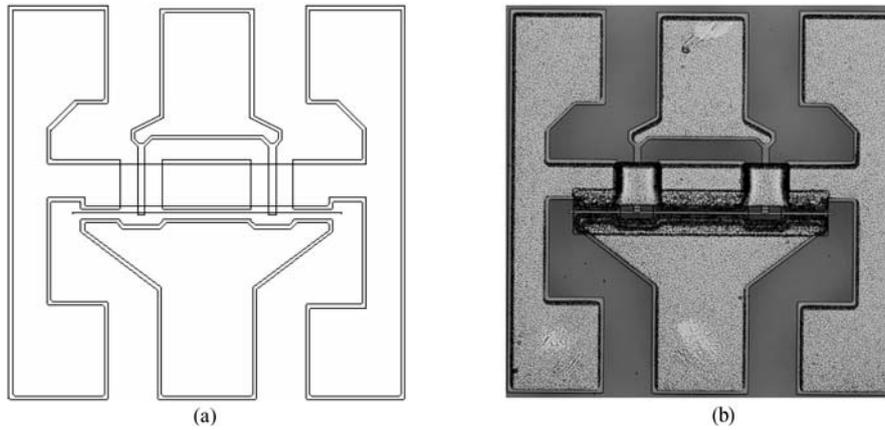
Fig. 2. (a) Layout and (b) top view micrograph of the low-noise GaN HEMT.
