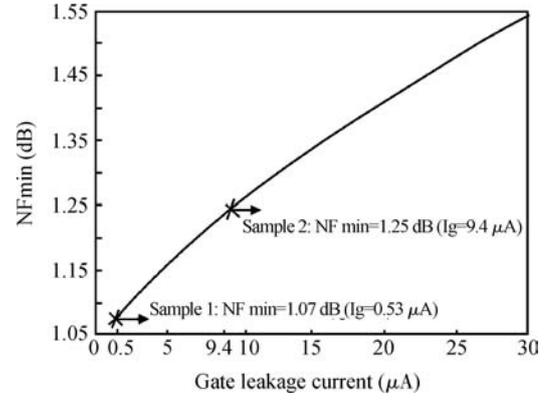
Fig. 6. Simulated minimum noise figure at 8 GHz with different gate leakage currents for GaN HEMTs.
