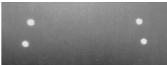
Fig. 3. Photograph showing the light emission from a 2 × 2 P+/N+/N-well light emitter array.
