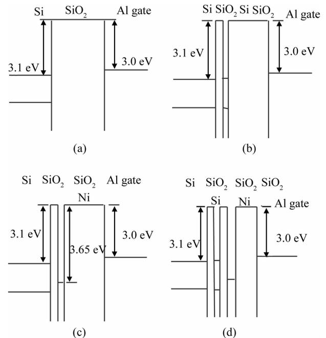
Fig. 3. Energy band diagrams of (a) control oxide, (b) Si nanocrystals, (c) Ni nanocrystals, and (d) Ni and Si nanocrystals.
