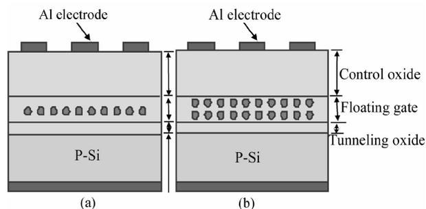
Fig. 1. Schematic cross-sectional structures of (a) MOS capacitor with single-layer semiconductor/metal nanocrystals and (b) MOS capacitor with double-layer semiconductor and metal nanocrystals.
