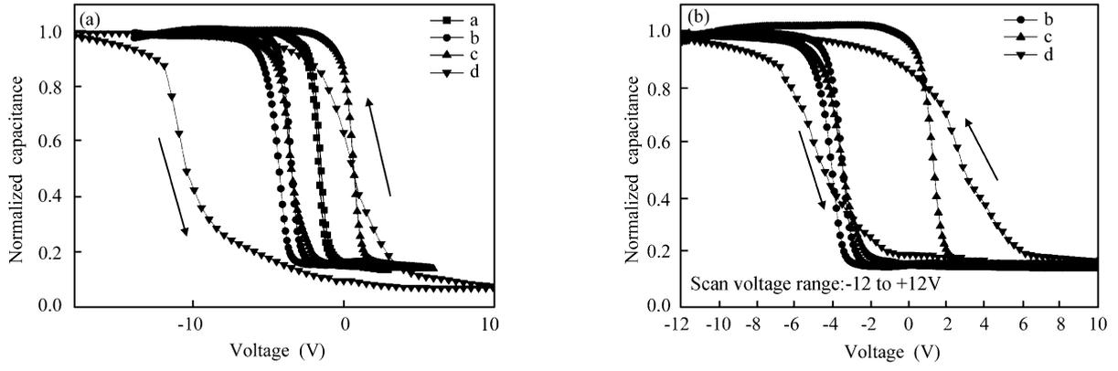
Fig. 4. High frequency  $C-V$  curves of MOS capacitors a–d in Table 1 at (a) different scanning voltage ranges and (b) the same scanning voltage ranges.
