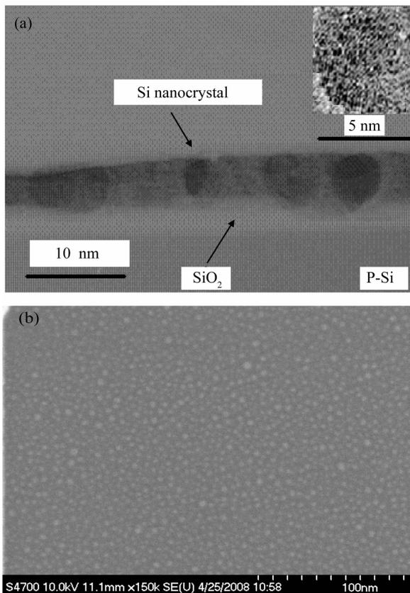
Fig. 2. (a) Typical TEM image of the MOS capacitor with single-layer Si nanocrystals; (b) Top view SEM image of Ni nanocrystals.
