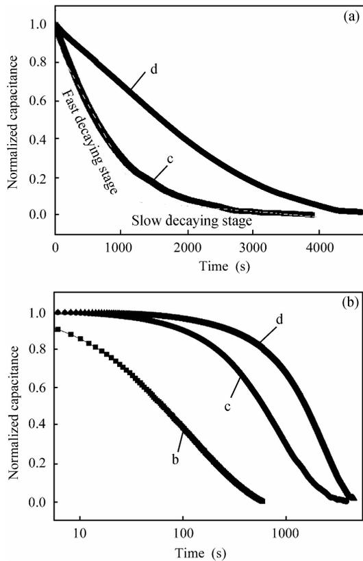
Fig. 5. Normalized capacitance versus time for MOS capacitor structures c and d in Table 1, where (a) and (b) correspond to linear and semi-logarithmic plots.
