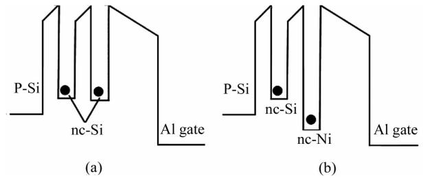
Fig. 6. Energy band diagrams of MOS capacitors with double-layer (a) homogeneous Si nanocrystals and (b) heterogeneous Si and Ni nanocrystals under retention.
