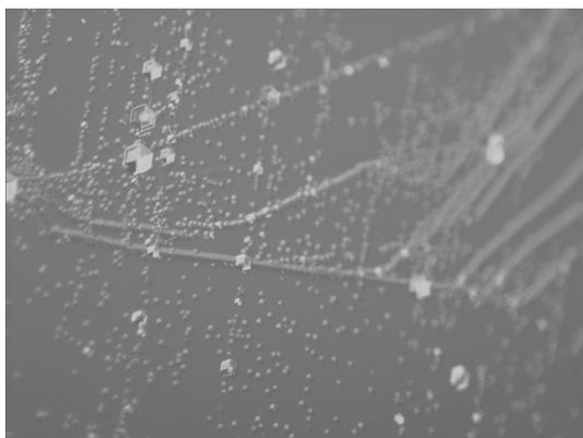
Fig. 1. Etching pits on a naturally formed (0001) Al surface of an AlN single crystal.
