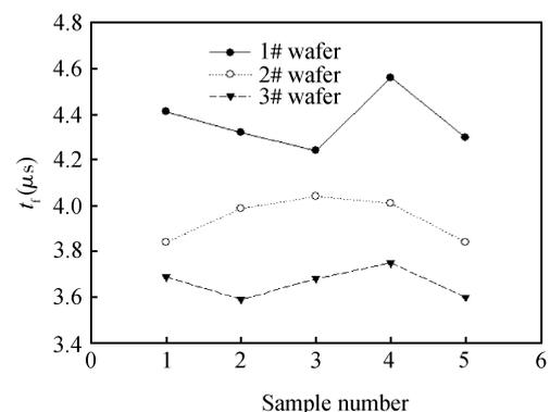
Fig. 1. Fall time of IGBT in different wafers before irradiation.
