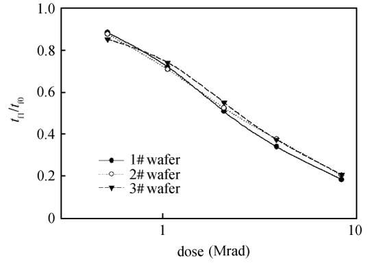
Fig. 3. Ratio of the fall time after irradiation to that before irradiation.
