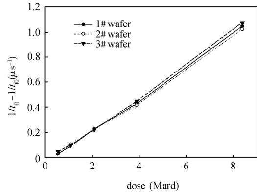
Fig. 4. Curves of  $1/t_{f1} - 1/t_{f0}$  versus dose in different wafers.
