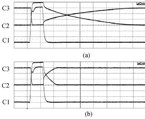
Fig. 2. Switching waveform of an IGBT (a) before and (b) after irradiation with a dose of 8 Mrad.
