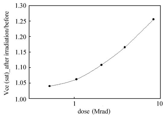
Fig. 5. Increase in the forward voltage drop with increasing radiation dose.
