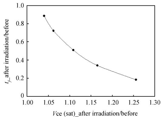
Fig. 6. Trade-off curve between the forward voltage drop and the fall time of an IGBT.
