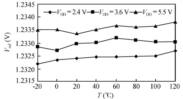
Fig. 8. Measured temperature dependence.
