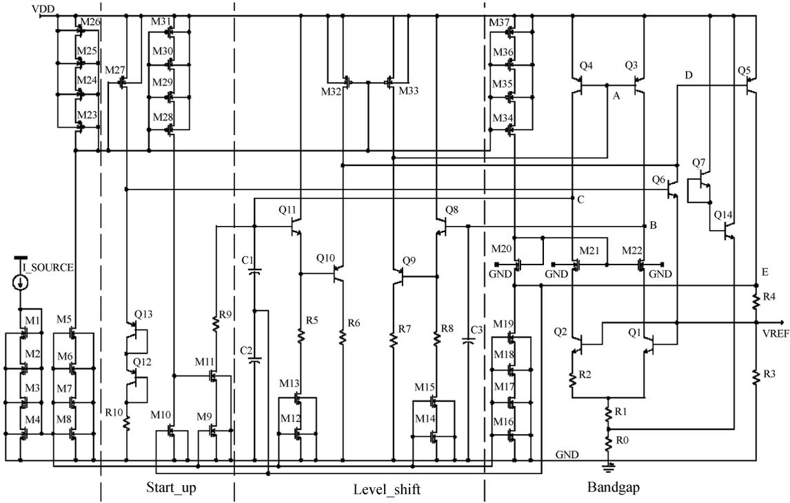
Fig. 3. Complete schematic of the proposed bandgap voltage reference.
