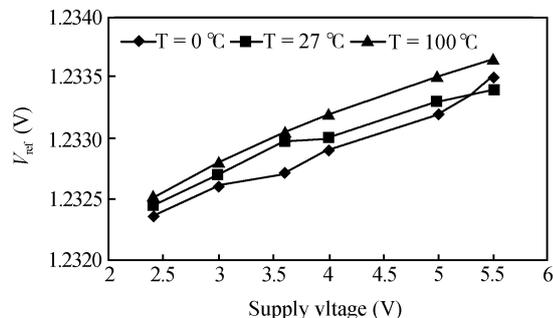
Fig. 9. Measured supply voltage dependence.
