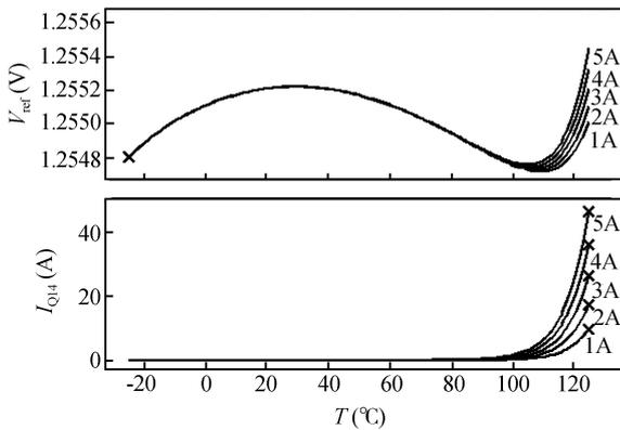
Fig. 5. Simulated TC of the proposed reference.
