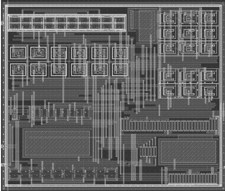
Fig. 4. Layout of the proposed bandgap voltage reference.
