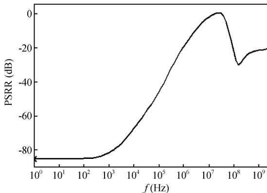
Fig. 6. Simulated PSRR of the proposed reference.
