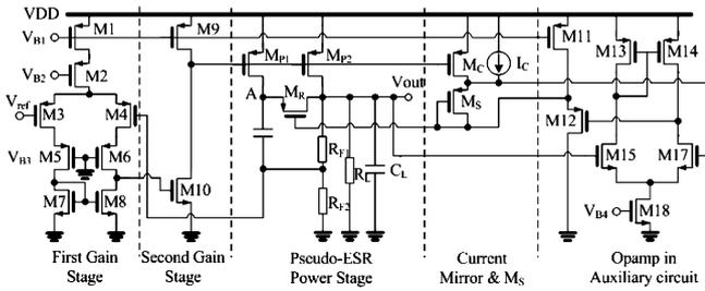
Fig. 13. Three-stage LDO based on pseudo-ESR power stage with controllable resistor.
