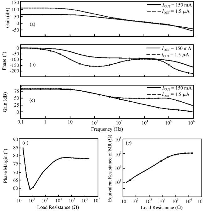
Fig. 7. AC simulation results of Miller capacitor compensation with controllable resistor under heavy load ( $I_{out} = 150 \text{ mA}$ ) and light load ( $I_{out} = 1.5 \mu\text{A}$ ): (a) Loop gain; (b) Loop phase; (c) Total gain of first and second gain stage; (d) Phase margin under all current load; (e) Equivalent Resistance of MR under all current load.
