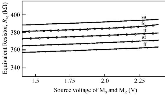
Fig. 5. Equivalent resistance of MR against the source voltage of MS and MR under process variation with 300 nA fixed copied current.
