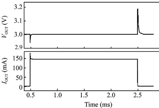
Fig. 15. Load regulation response of the LDO when  $I_{OUT}$  changes between 1.5 A and 150 mA for the LDO with pseudo-ESR power stage.
