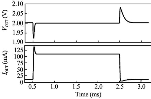
Fig. 11. Load regulation response of LDO when  $I_{OUT}$  changing between 10 mA and 100 mA for UGCC LDO.
