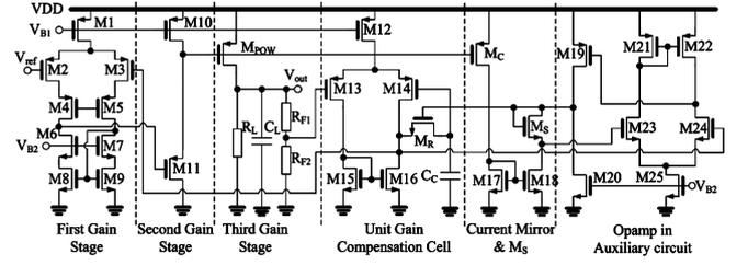
Fig. 9. Three-stages LDO based on unit gain compensation cell with controllable resistor.
