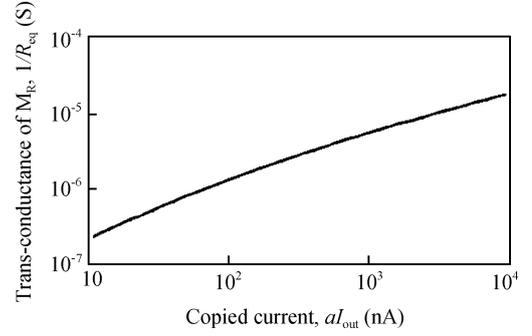
Fig. 4. Trans-conductance of MR,  $1/R_{eq}$ , against the copied current.
