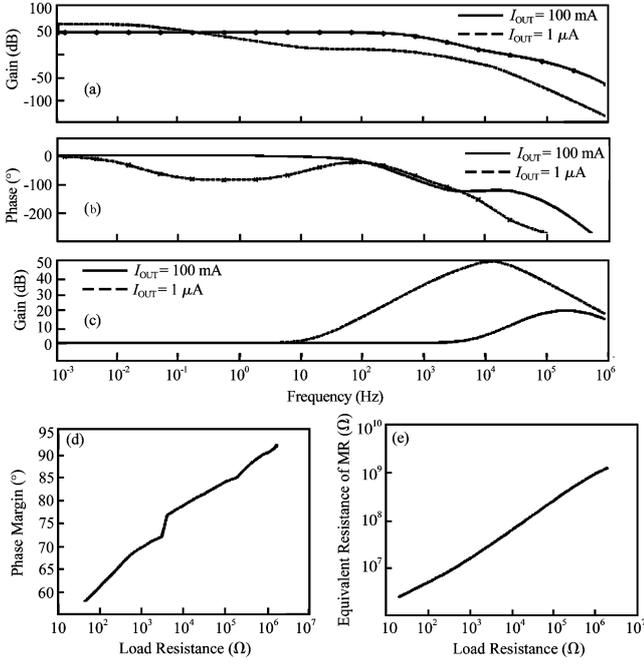
Fig. 10. AC simulation results of UGCC with controllable resistor under heavy load ( $I_{out} = 100$  mA) and light load ( $I_{out} = 1$   $\mu$ A): (a) Loop gain; (b) Loop phase; (c) Gain of UGCC; (d) Phase margin under all current load; (e) Equivalent resistance of MR under all current loads.
