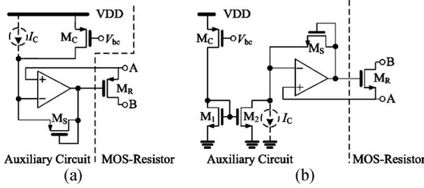
Fig. 2. Controllable resistor with auxiliary circuit, assuming that the current to be proportional is generated by a PMOS: (a) for P-type MOS-resistor; (b) for N-type MOS-resistor.
