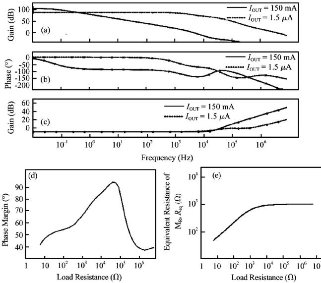
Fig. 14. AC simulation results of pseudo-ESR power stage with controllable resistor under heavy load ( $I_{out} = 100 \text{ mA}$ ) and light load ( $I_{out} = 1 \mu\text{A}$ ): (a) Loop gain; (b) Loop phase; (c) Gain of UGCC; (d) Phase margin under all current load; (e) Equivalent resistance of MR under all current load.
