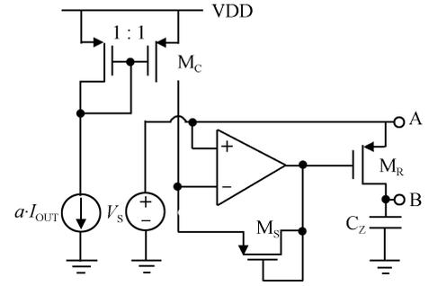
Fig. 3. Testing circuit for the controllable resistor.
