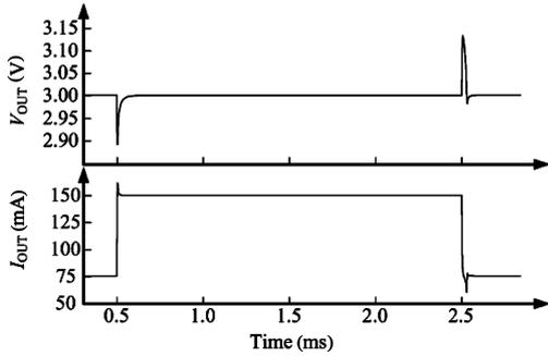
Fig. 8. Load regulation response of the LDO when  $I_{out}$  changes between 75 mA and 150 mA for SMCNR LDO.
