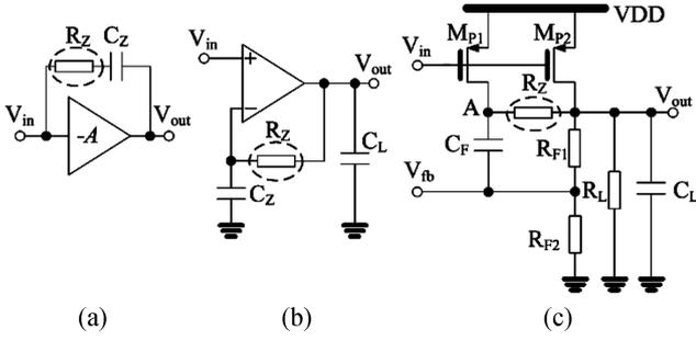
Fig. 1. Zero generation circuits,  $R_z$  in the dashed ellipse is the corresponding resistor used to generate the zero. (a) Single Miller capacitor with nulling resistor; (b) Unit gain compensation cell; (c) Pseudo-ESR power stage.
