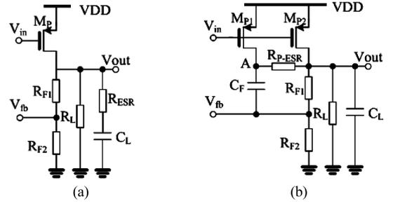
Fig. 12. (a) Traditional ESR circuit; (b) Power stage and feedback network with pseudo-ESR.
