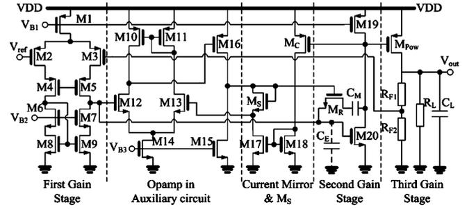
Fig. 6. Three-stage LDO with Miller capacitor frequency compensation, and the nulling resistor is controllable to form a tracking zero by the auxiliary circuit.
