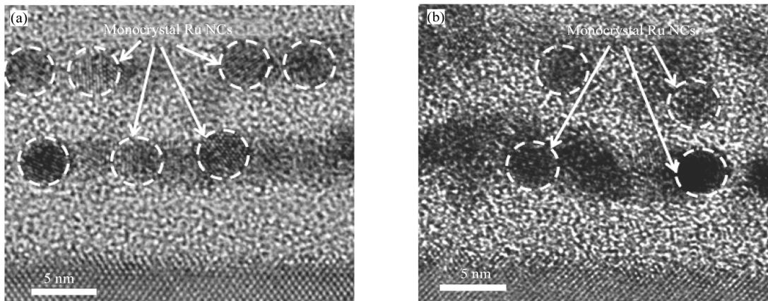
Fig. 2. Cross-sectional HRTEM images of stacked Ru NCs formed by two methods: (a) Sample A is by RTA (900 °C, 30 s) for the whole gate stacks; (b) Sample B is by RTA (600 °C, 1 min) before each SiO<sub>2</sub> deposition.
