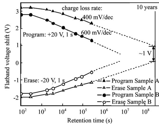
Fig. 5. Retention performance of stacked Ru NC MOS capacitors fabricated by the two methods.
