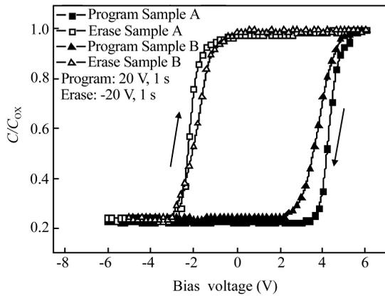
Fig. 3. Capacitance–voltage ( $C$ – $V$ ) characteristics for samples A and B. The amplitude and width of the voltage pulse are  $\pm 20$  V and 1 s for the program and erase state respectively.
