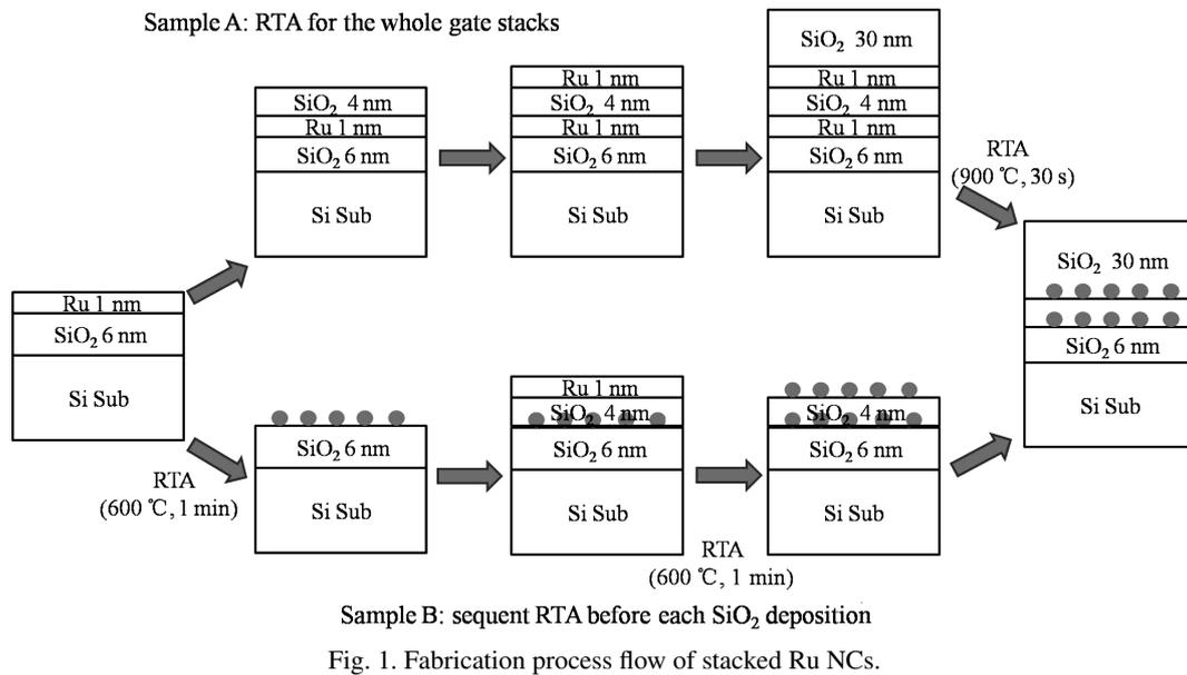
Fig. 1. Fabrication process flow of stacked Ru NCs.
