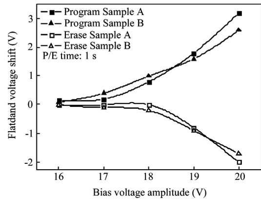
Fig. 4. Flatband voltage shifts of Ru NCs capacitors under various P/E operations.
