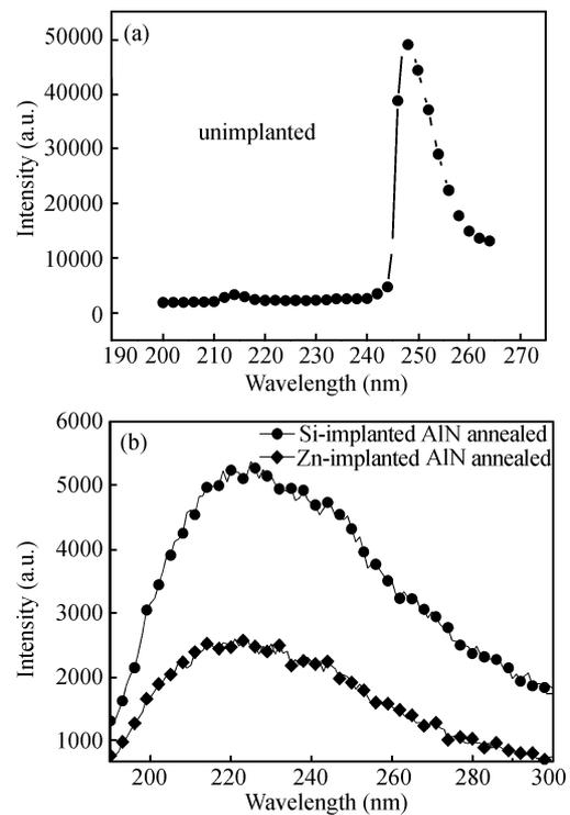
Fig. 2. PL spectra of AlN single crystal: (a) Original AlN; (b) Si- and Zn-implanted and annealed.
