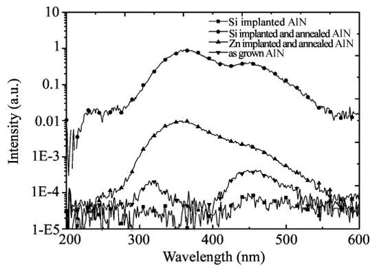
Fig. 1. CL spectra of as-grown undoped AlN single crystal and AlN single crystals implanted with Si and Zn.
