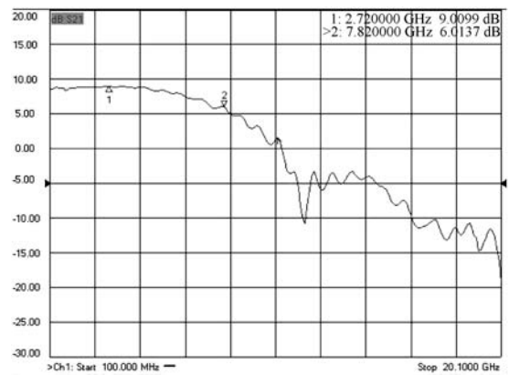
Fig. 4. Small signal S parameter of the current mode TIA.
