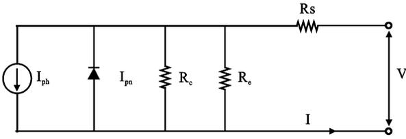
Fig. 2. Equivalent circuit for the new structure solar cell.  $R_c$  is the shunt resistance caused by the penetration of front contacts fingers through the p–n junction, and  $R_e$  is by the other shunting in the emitter except  $R_c$ .
