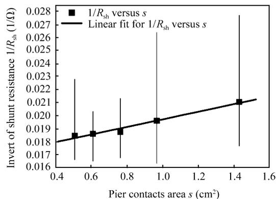
Fig. 5. Relation between the area of pier contacts  $s$  and the inverse of solar cell shunt resistances  $1/R_{sh}$ . The linear fitting for  $1/R_{sh}$  versus  $s$  is also shown.
