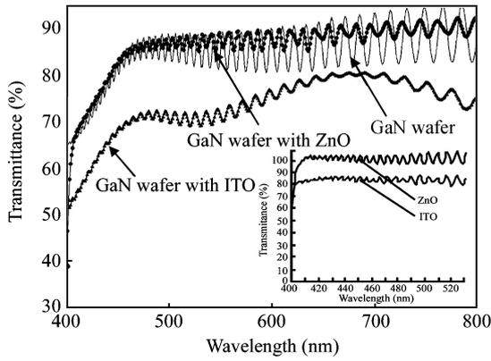
Fig. 3. Transmittance spectra of ZnO (~8  $\mu\text{m}$ ) and ITO (~200 nm) on GaN.
