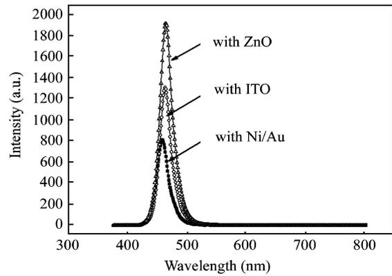
Fig. 5. EL spectra of LEDs with ZnO, ITO, and Ni/Au current spreading layers at 20 mA.
