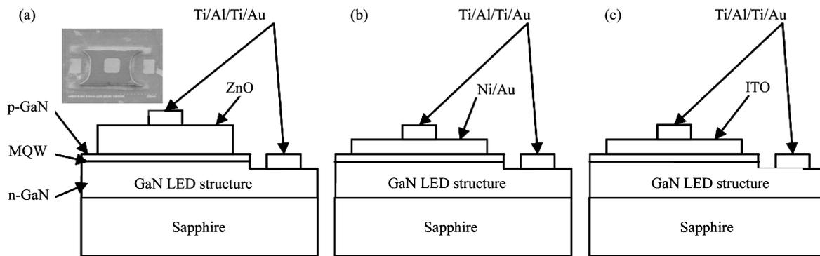
Fig. 1. Schematic structure of the GaN-based LEDs with (a) ZnO (8  $\mu\text{m}$ ), (b) Ni/Au (5 nm/5 nm), and (c) ITO (200 nm) as the transparent electrode.
