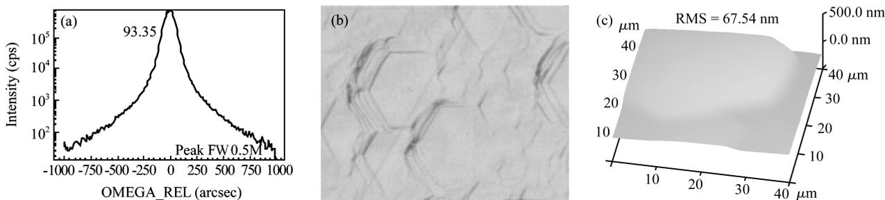
Fig. 2. Characteristics of the ZnO layers: (a) Rocking curve of ZnO (002); (b) Microscopic image of the ZnO surface; (c) AFM views of the ZnO surface.
