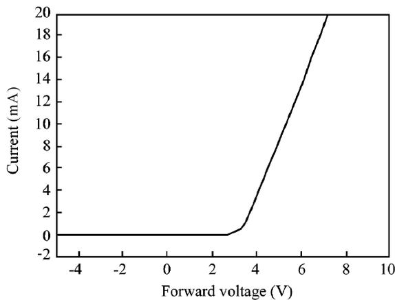
Fig. 7.  $I$ - $V$  characteristics of the LED with a ZnO transparent layer.
