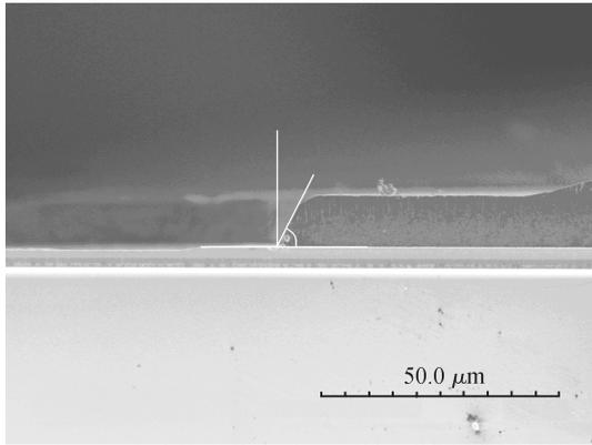
Fig. 4. SEM picture of the cross section of an etched ZnO film.
