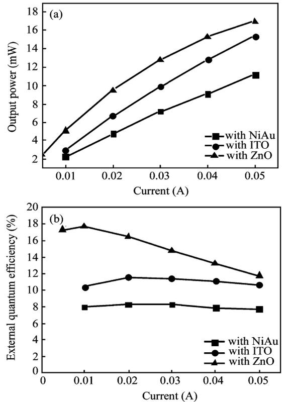
Fig. 6. (a) Output power and (b) external quantum efficiency of GaN-based LEDs with Ni/Au, ITO, and ZnO current spreading layers at forward currents from 5 to 50 mA.
