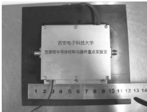
Fig. 8. External view of the one-way GaN HEMT amplifier.
