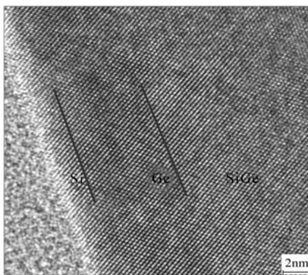
Fig. 4. High resolution XTEM image of the Si/Ge/SiGe interface of the strained Ge sample. No dislocation nucleation has been observed at the Si/Ge/SiGe interfaces.
