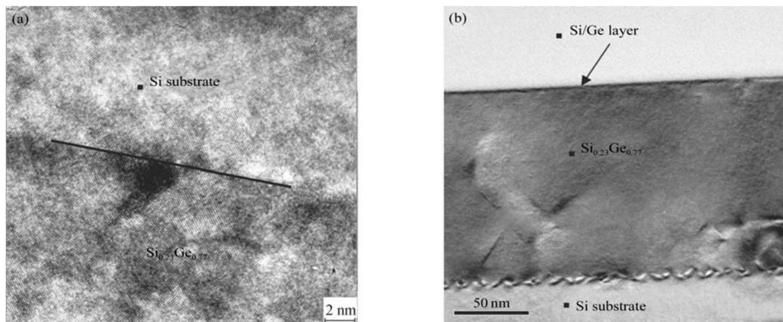
Fig. 5. (a) High resolution XTEM image of the SiGe/Si substrate interface; (b) XTEM image of the whole epitaxial layer including the Si cap/Ge/SiGe/Si substrate. Many dislocations nucleate at the SiGe/Si substrate interface and extend into the SiGe layer at an angle of  $60^\circ$  with the interface, but most of them are terminated in the SiGe layer by interacting with each other.
