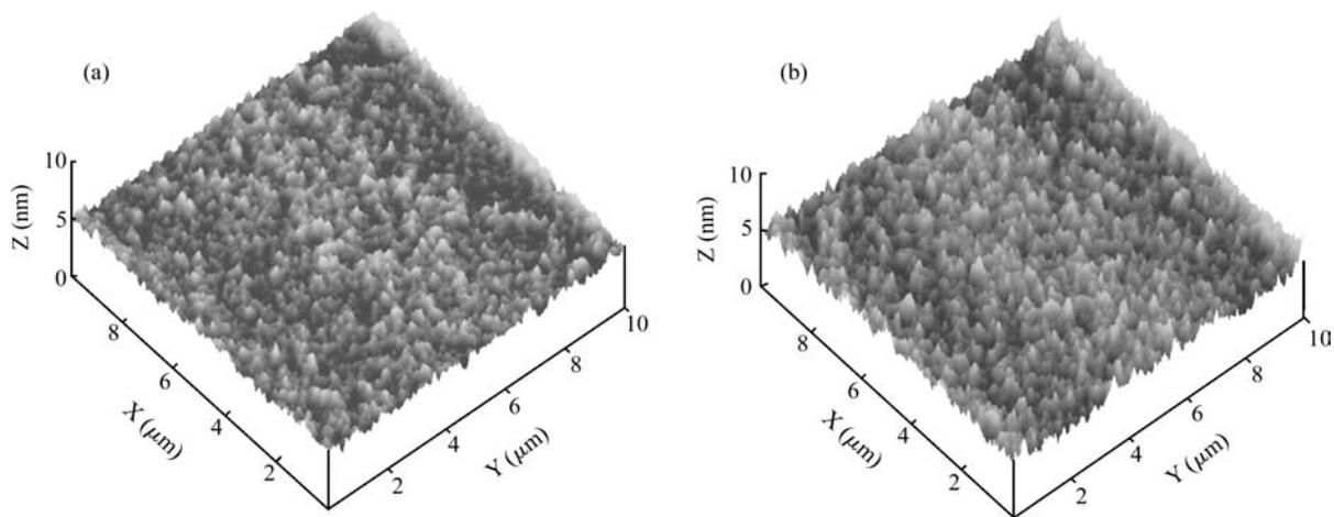
Fig. 3. AFM images of sample surfaces after (a) growth of the SiGe virtual substrate layer, RMS = 0.3 nm, (b) growth of the strained Ge layer and Si passivation layer, RMS = 0.4 nm.
