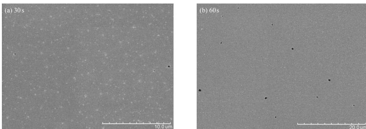
Fig. 6. Surface SEM images of the strained Ge sample etched by diluted Schimmel solution with different etching times: (a) 30 s; (b) 60 s. The black pits in the images represent the threading dislocations running through to the surface.
