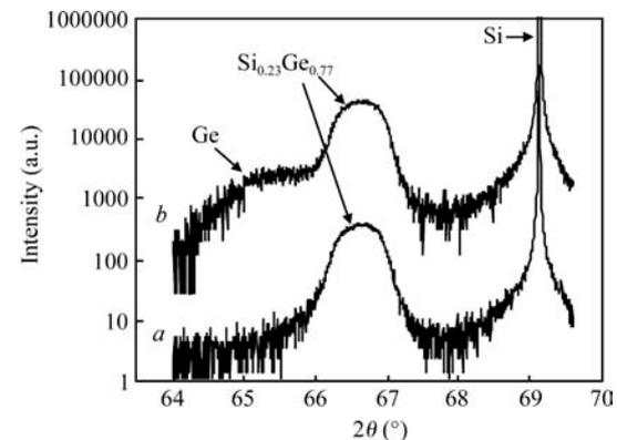
Fig. 2. DCXRD  $\omega$ - $2\theta$  curves of the (004) planes of samples after (a) growth of the SiGe virtual substrate layer and (b) growth of the strained Ge layer and Si cap layer.
