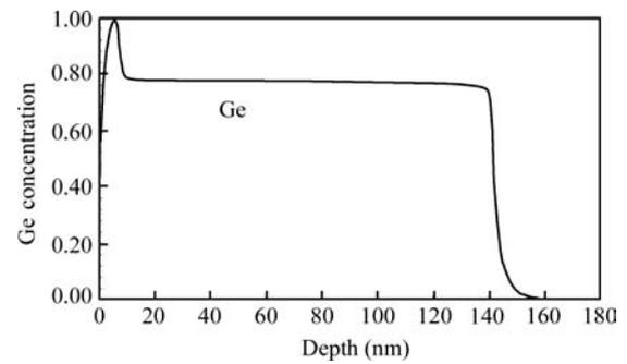
Fig. 1. SIMS curve of the strained Ge sample.
