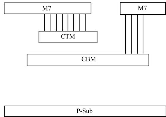
Fig. 3. Side view of MIM capacitor without concave shield.
