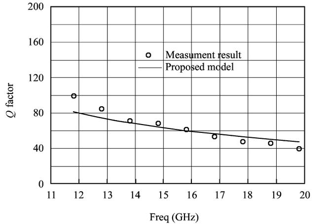
Fig. 7.  $Q$  factor of proposed model and measurement result.
