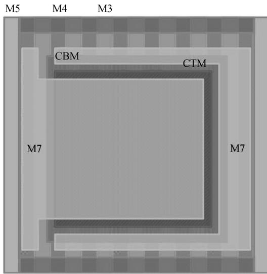
Fig. 1. Top view of MIM capacitor with concave shield.
