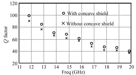
Fig. 5.  $Q$  factor of MIM capacitor.
