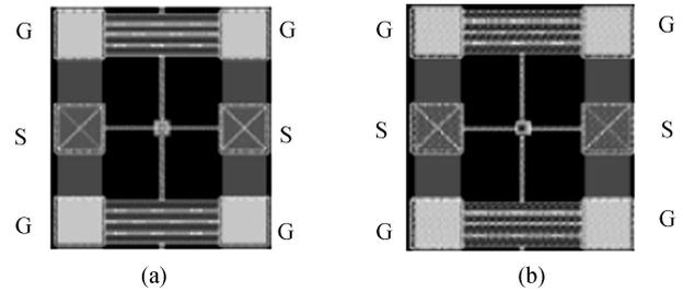
Fig. 4. GSG test structure of MIM capacitor (a) with concave shield and (b) without concave shield.
