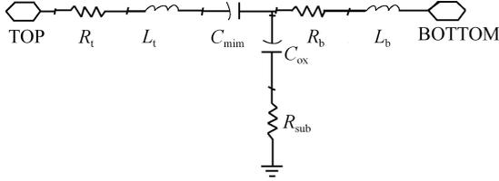
Fig. 6. Circuit model of MIM capacitor with concave shield.
