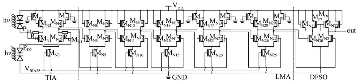
Fig. 3. A standard CMOS, fully differential optoelectronic integrated receiver with MSM photodetector.
