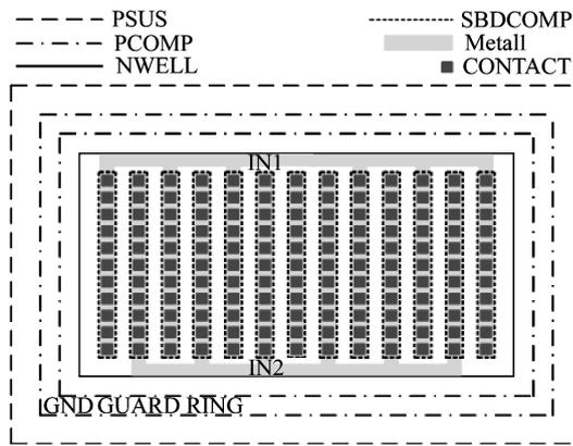
Fig. 2. A standard CMOS MSM photodetector based on the Metal1-NWELL Schottky diode.
