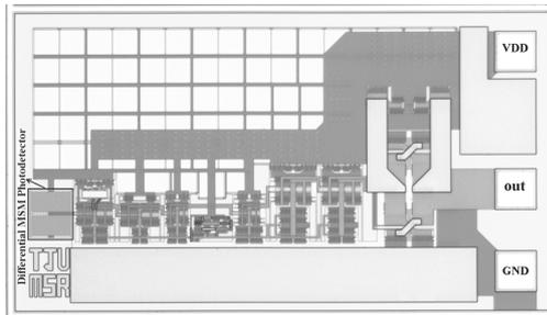
Fig. 4. Die photograph of the optoelectronic integrated receiver in a chartered 0.35  $\mu\text{m}$ , 3.3 V standard CMOS process.
