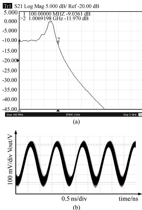
Fig. 5. Measured results: (a) Optic frequency response for 850 nm wavelength with  $-10$  dBm optical power; (b) Transient response at 1 GHz for 850 nm wavelength with  $-10$  dBm optical power.
