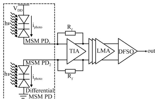
Fig. 1. A fully differential optical receiver with integrated MSM photodetector.
