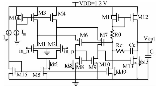
Fig. 4. Schematic of a low-voltage low-power amplifier.
