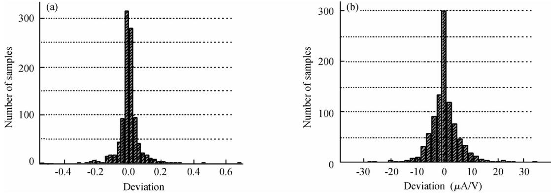
Fig. 3. Model deviation histograms for (a)  $r$  and (b)  $g_m$ .
