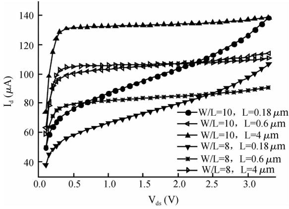
Fig. 1. Output characteristic curves of NMOS obtained from BSIM3v3 device models ( $V_{gs} = 0.7$  V,  $V_{sb} = 0$ ).
