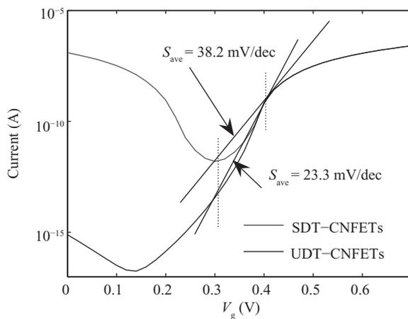
Fig. 8. The transfer characteristics of UDT-CNFETs (gray line) and SDT-CNFETs (black line) with  $V_{DS} = 0.6$  V,  $a = c = 15$  nm,  $b = 30$  nm,  $\rho_1 = 4 \times 10^8$  m $^{-1}$ ,  $\rho_2 = 4 \times 10^6$  m $^{-1}$ .
