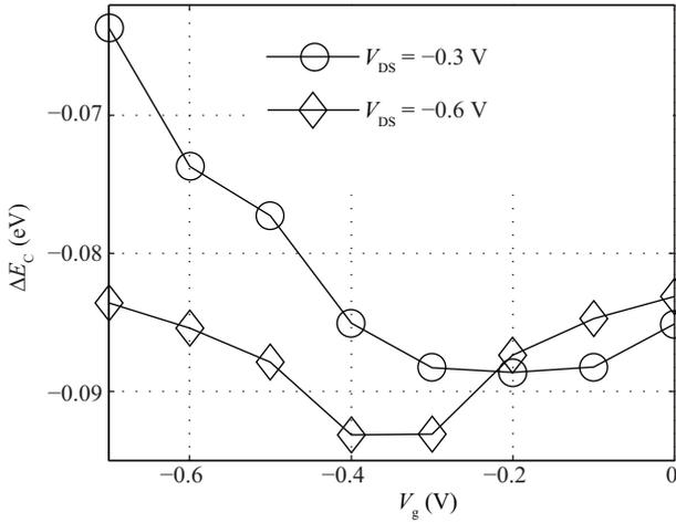
Fig. 3. Impact of quantum capacitance on the CNT surface potential in T-CNFETs with  $V_{DS}$  of  $-0.3$  V (circle-marked line) and  $-0.6$  V (diamond-marked line).
