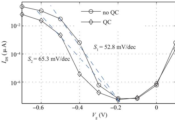
Fig. 4. Impact of quantum capacitance on the transfer characteristic of T-CNFETs with  $V_{DS} = -0.6$  V.
