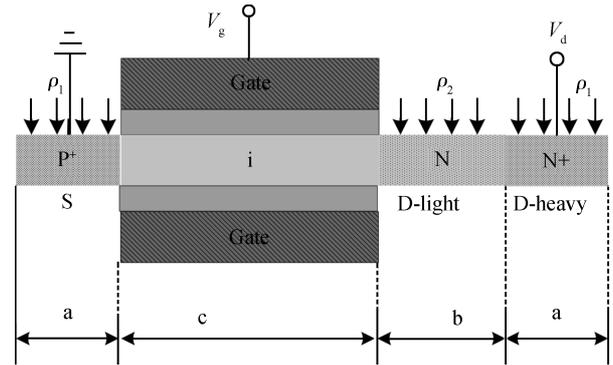
Fig. 7. Two-dimension sketch of the SDT-CNFET device structure.
