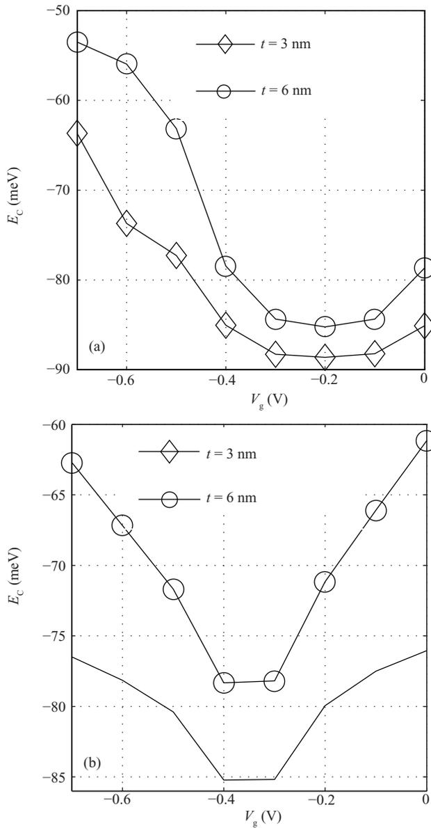
Fig. 6. Impact of insulator thickness on the CNT surface potential in T-CNFETs with  $V_{DS}$  of  $-0.3$  V (circle-marked line) and  $-0.6$  V (diamond-marked line).
