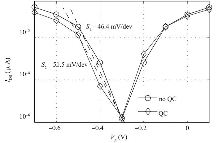
Fig. 5. Impact of quantum capacitance on the transfer characteristic of T-CNFETs with  $V_{DS} = -0.3$  V.
