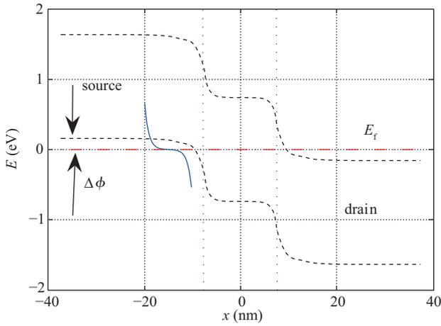
Fig. 1. T-CNFET band diagram, where gate voltage  $V_g = 0$  V, drain-source bias voltage  $V_{DS} = 0$  V, source/drain doping level  $\rho = 8 \times 10^8$   $\text{cm}^{-1}$ , tight-binding parameter  $\phi_{pp} = -3$  eV, insulator thickness  $t = 2$  nm, insulator dielectric constant  $\epsilon = 16$ .
