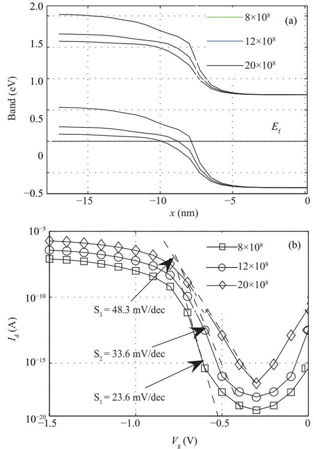
Fig. 2. (a) Impact of doping level on band structure in T-CNFETs, and (b) the corresponding transfer characteristics with  $V_{DS} = -0.6$  V.
