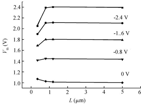
Fig. 3. Threshold voltage versus channel length for SOI nMOSFETs with different  $V_{ps}$ .
