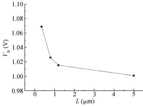
Fig. 2. Threshold voltage versus channel length for an SOI nMOSFET.
