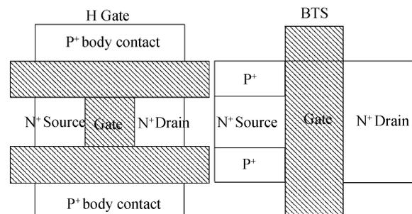
Fig. 1. Layout of H-gate and BTS nMOSFETs.
