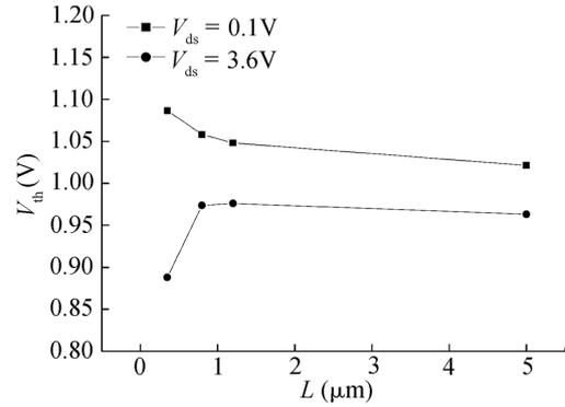
Fig. 5. Threshold voltage versus channel length for SOI nMOSFETs with different  $V_{ds}$ .
