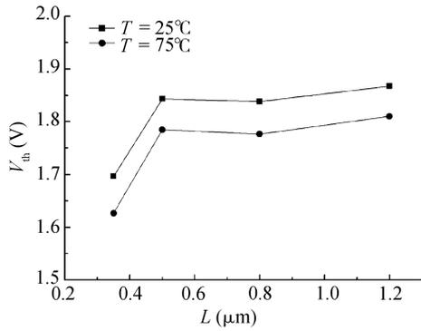
Fig. 6. Threshold voltage versus channel length at different temperatures.
