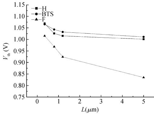
Fig. 7. Threshold voltage versus channel length for body contact and floating body SOI nMOSFETs.
