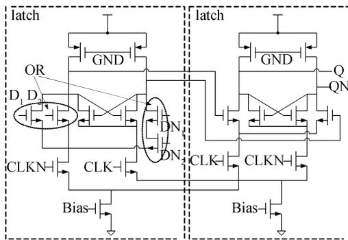
Fig. 4. Schematic of CML D flip-flop with merged OR gate.
