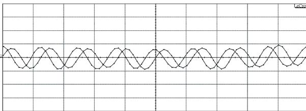
Fig. 10. Measured output waveforms of the I and Q channels (200 ps/div, 50 mV/div).
