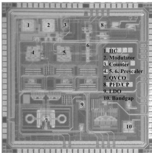
Fig. 7. Microphotograph of the frequency synthesizer.
