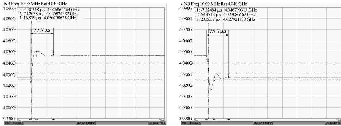
Fig. 9. Measured settling transient response.
