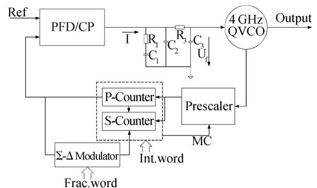
Fig. 1. Fractional- $N$  frequency synthesizer architecture.
