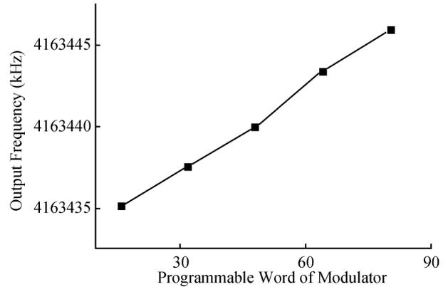
Fig. 8. Measured output frequency versus programmable word of modulator.
