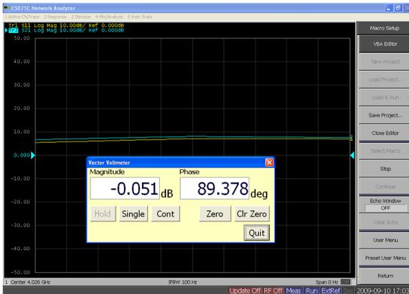
Fig. 11. Measured output amplitude and phase difference of the I and Q channels.
