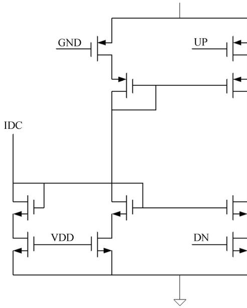
Fig. 6. Schematic of CP.
