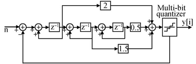
Fig. 5. Equivalent model of  $\Sigma$ - $\Delta$  modulator.
