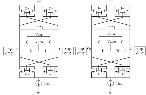
Fig. 2. Schematic of LC-tank QVCO.
