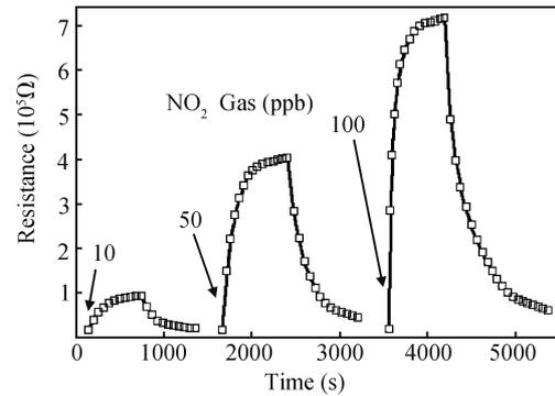
Fig. 5. Resistance changes of sensor as a function of time for three cycles of a sequence of NO<sub>2</sub> concentrations ranging from 10 to 100 ppb.
