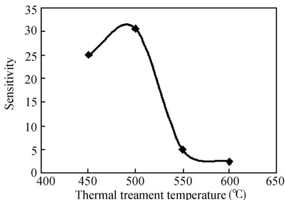
Fig. 8. Relationship between sensitivity of sensor versus temperature of thermal treatment on 100 ppb NO<sub>2</sub>.
