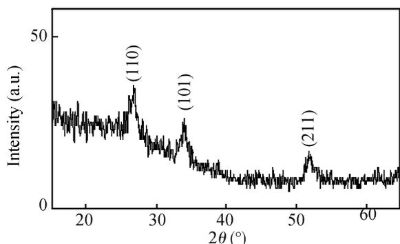
Fig. 1. XRD patterns of SnO<sub>2</sub>/MWCNT material.
