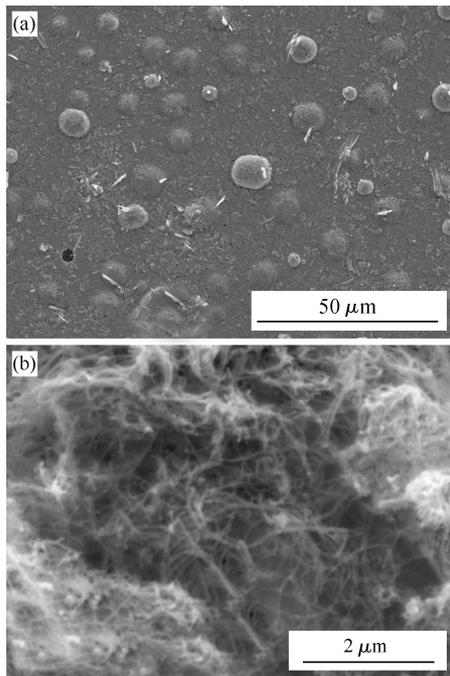
Fig. 3. SEM image of MWCNT-doped SnO<sub>2</sub> and enlarged partial image.
