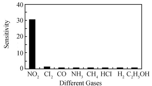
Fig. 6. Selectivity property of sensor and its sensitivity to 100 ppb NO<sub>2</sub> versus another gas of 100 ppm.
