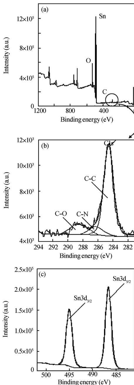
Fig. 2. XPS patterns of MWCNT-doped SnO<sub>2</sub> thin film material of (a) survey, (b) C1s, and (c) Sn3d.
