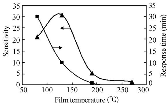
Fig. 7. NO<sub>2</sub> sensitivity (100 ppb) and response time versus temperature of film of sensor.
