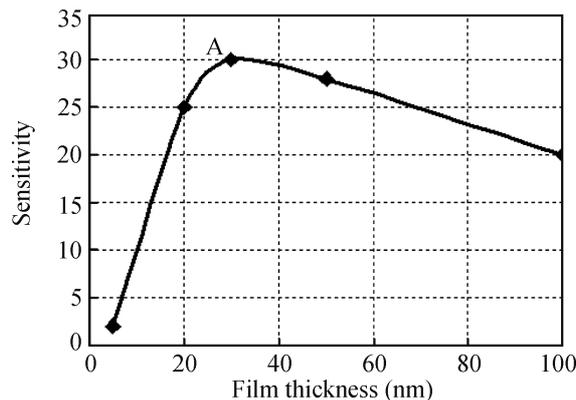
Fig. 9. Effect of film thickness of gas sensor versus sensitivity on 100 ppb NO<sub>2</sub>.
