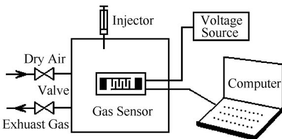
Fig. 4. Schematic diagram of apparatus for measuring gas sensor property.
