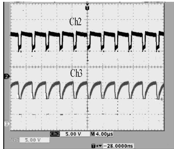
Fig. 11. Test result of traditional and improved drive circuit for a P-channel power MOSFET.
