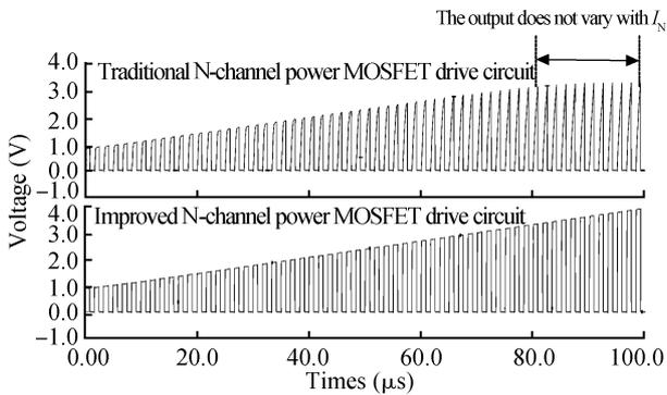
Fig. 9. Variation of output for an N-channel power MOSFET.
