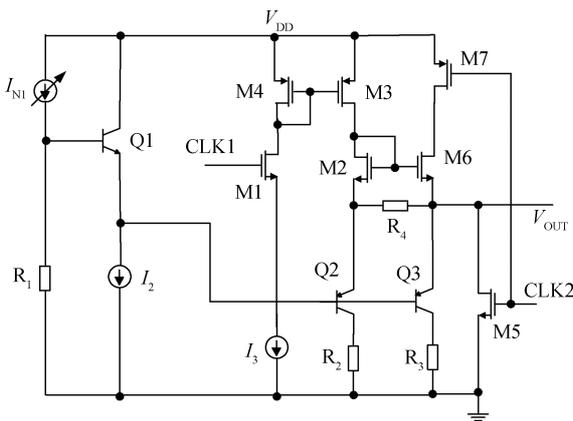
Fig. 5. Improved drive circuit for an N-channel power MOSFET.
