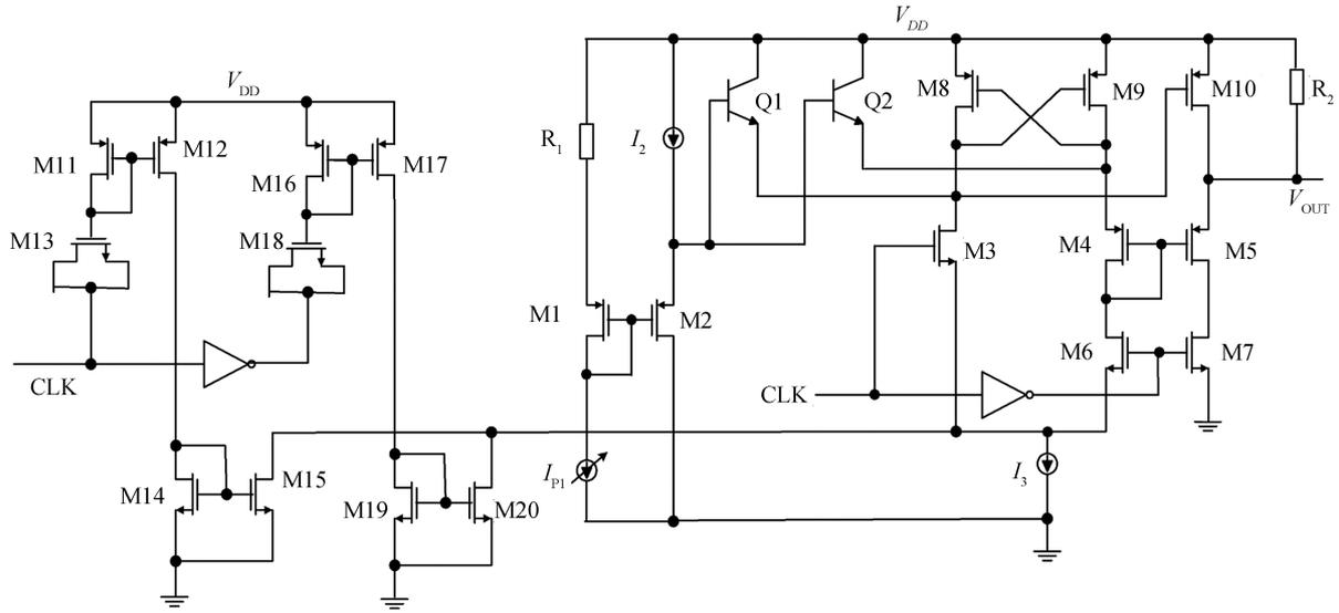
Fig. 3. Improved drive circuit for a P-channel power MOSFET.
