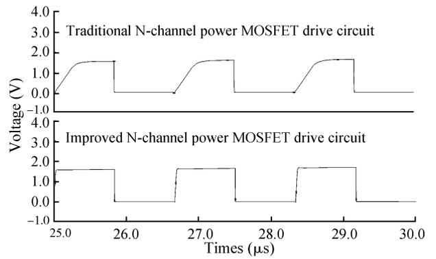
Fig. 10. Transient response of drive circuit for an N-channel power MOSFET.
