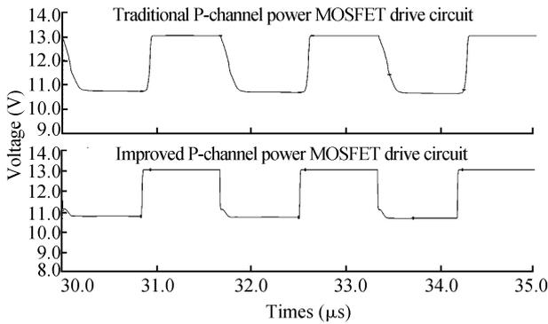
Fig. 8. Transient response of drive circuit for a P-channel power MOSFET.
