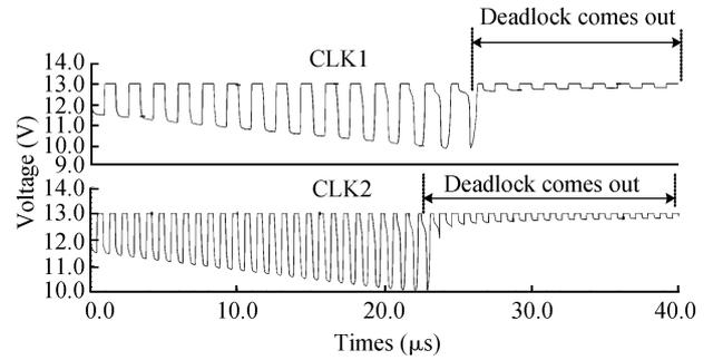
Fig. 6. Variation of deadlock with frequency for a P-channel power MOSFET.
