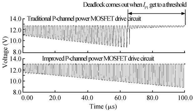
Fig. 7. Variation of output for a P-channel power MOSFET.
