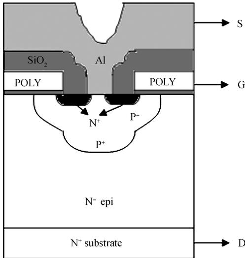
Fig. 1. Cross-section view of VDMOS structure[5].
