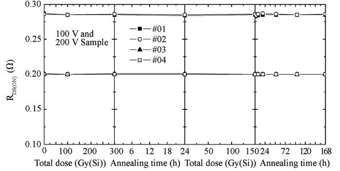
Fig. 8. On-state resistance of devices #01, #02, #03 and #04 versus total dose and annealing time.
