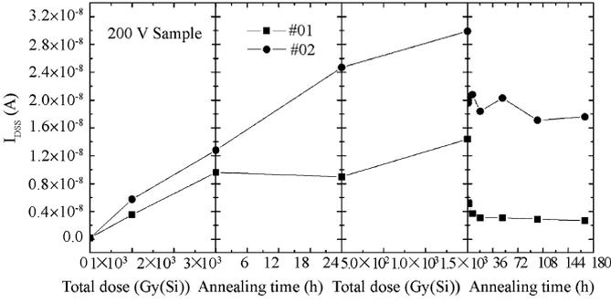
Fig. 6. Drain current of devices #01, #02 versus total dose and annealing time.
