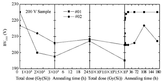
Fig. 4. Breakdown voltage of devices #01, #02 versus total dose and annealing time.
