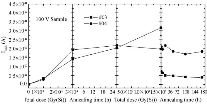
Fig. 7. Leakage current of devices #03, #04 versus total dose and annealing time.
