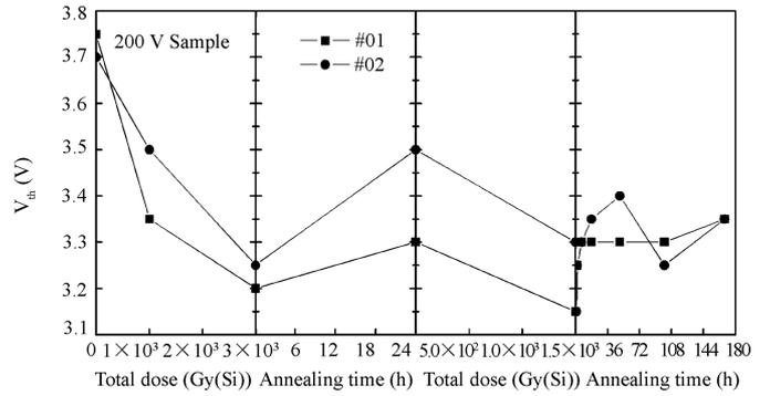
Fig. 2. Threshold voltage of devices #01, #02 versus total dose and annealing time.
