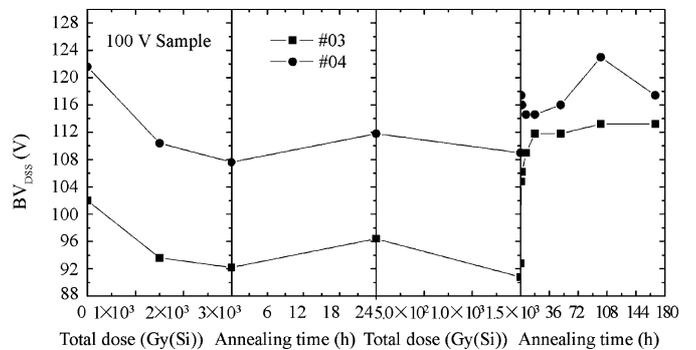
Fig. 5. Breakdown voltage of devices #03, #04 versus total dose and annealing time.
