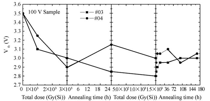
Fig. 3. Threshold voltage of devices #03, #04 versus total dose and annealing time.
